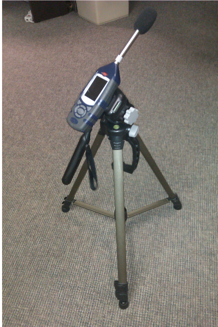
Figure 3.3: Image describing the set-up of the sound level meter used for noise exposure assessment. Not shown: AC adapter used to power the device.
