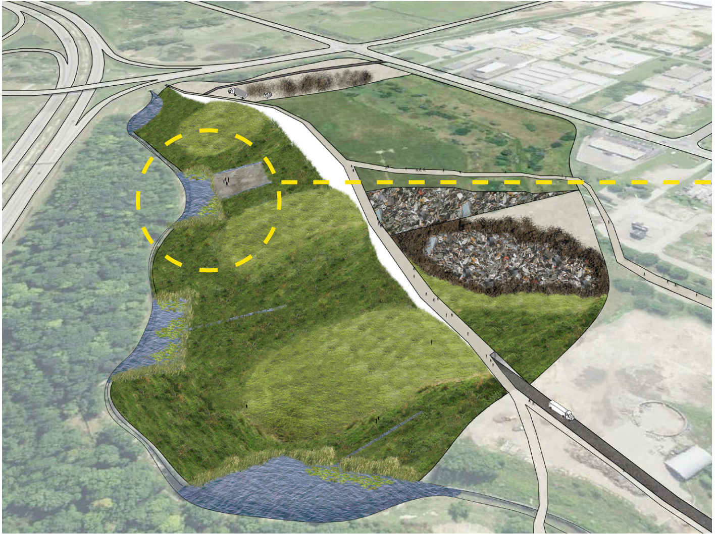
fig. 6.36 Aerial view of final landfill mining, secondary sanitary landfill creation, and landscape intervention on The Upper Ottawa Street Landfill
