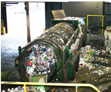
fig. 3.04 a trommel screen sorting recyclable goods in an MRF
