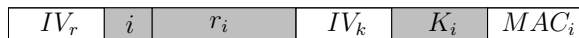
Figure 3.2: The layout of a data item. The light grey parts are encrypted.
