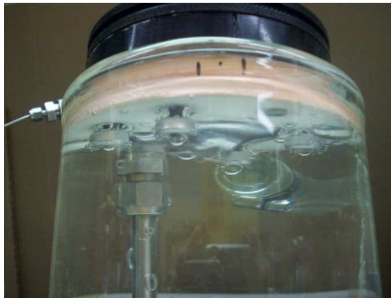
Figure 3-8: Bubble formation at the surface of the membrane
