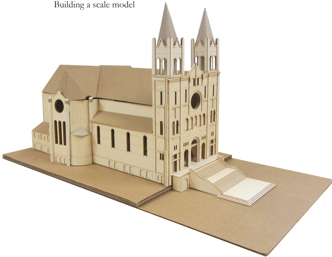
Fig.3.26. Model (1:100) of the church. Materials used: taskboard and cardboard.
