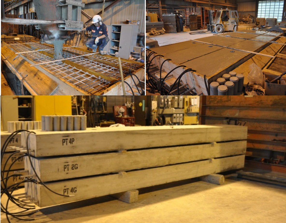
Figure 3.13 - Pouring concrete and completed specimens following formwork removal
