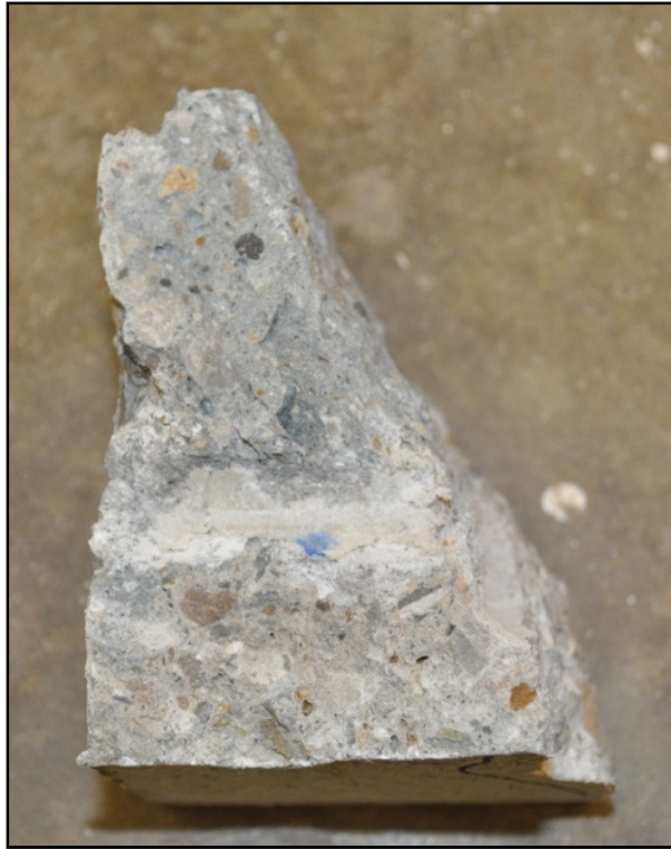
Figure 5.25 - White residue from the GFRP bar surface remains on the concrete after testing
