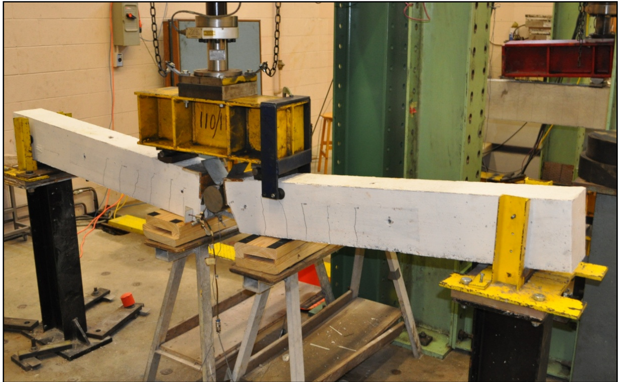
Figure 5.23 - Beam-hinge specimen post-failure
