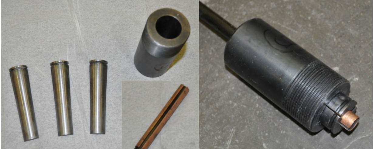
Figure 2.3 - CFRP split wedge anchor system
