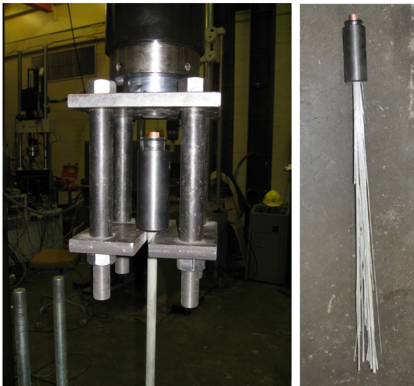
Figure 5.6 - GFRP bar uniaxial tension test
