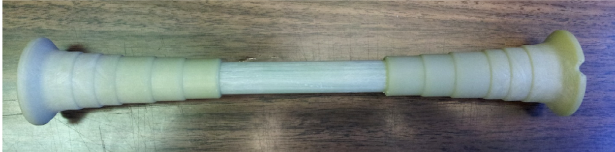
Figure 3.4 – Double-headed shear bar used for Phase III
