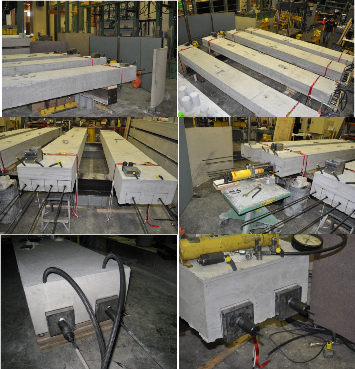
Figure 3.16 - Slabs before and after prestressing
