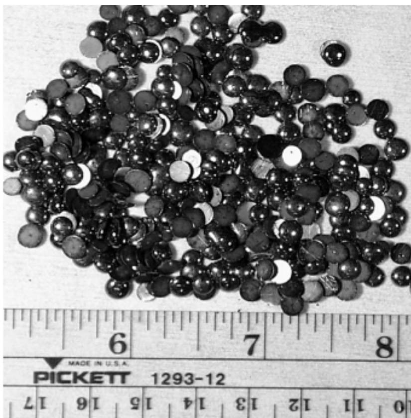
Figure 2.11: Stabilized selenium tablets with Arsenic doping and Chlorine used for fabrication of uniform a-Se films via vacuum evaporation technique[3].
