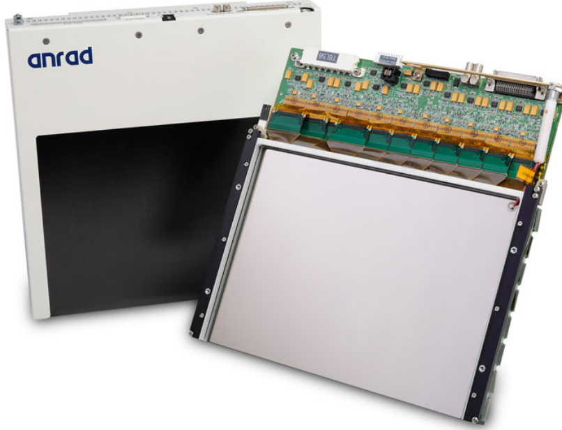
Figure 2.10: Commercial a-Se semiconductor direct x-ray detector for full-field digital mammography (FFDM).
