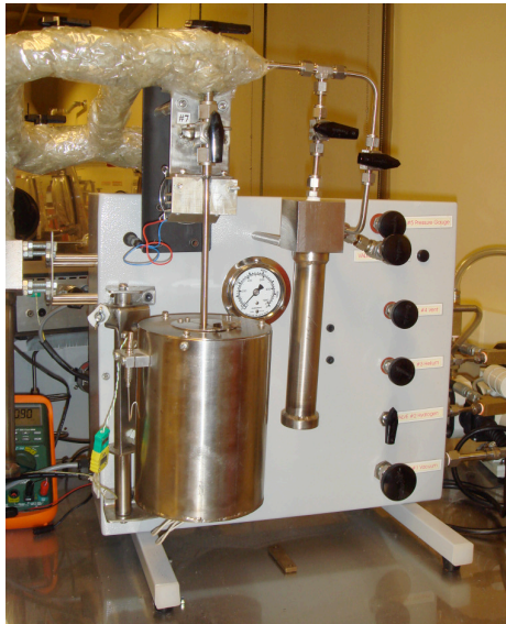
Fig. 3.2 A Sieverts-type apparatus custom-built by A.O.C. Scientific Engineering Pty Ltd., Australia, for evaluating hydrogen storage properties.
