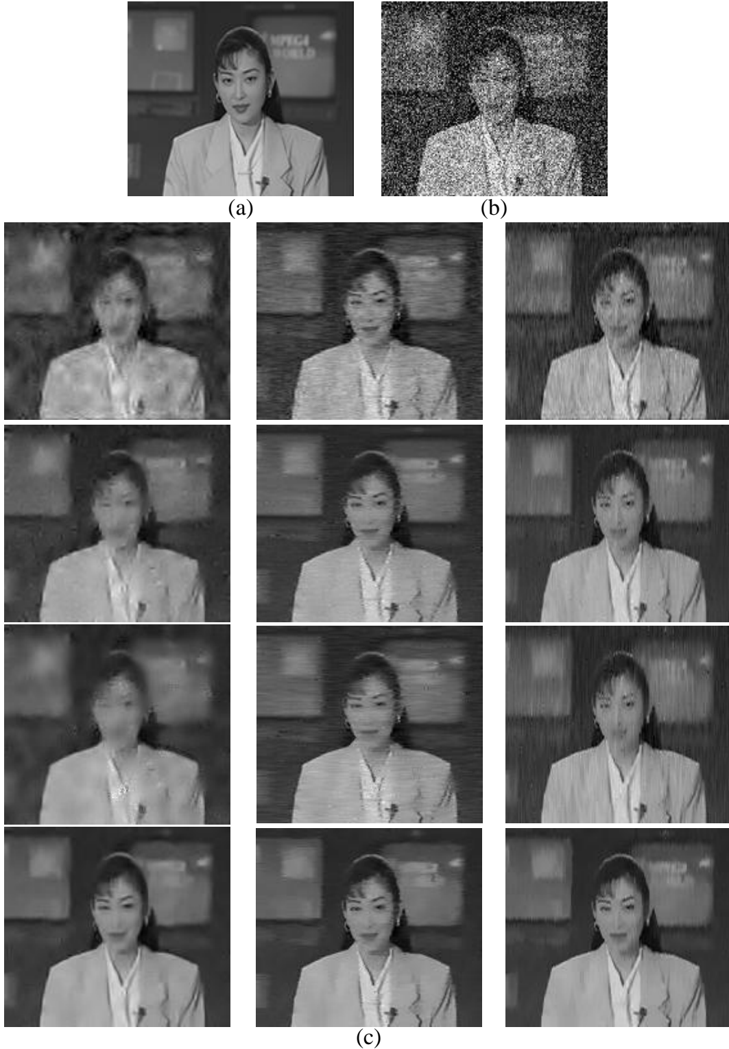
Figure 5.2: Denoised frames from three different views using different denoising algorithms. (a) Original frame; (b) Noisy frame with \sigma_n = 50 ; (c) Top to bottom: denoised frames by SURE-LET, BLS-GSM, K-SVD, and VBM3D; Left to right: denoised frames from front-, top-, and side-views, respectively.
