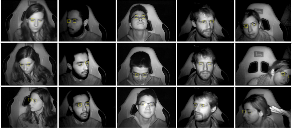
Figure 5.3: Example of tracking results for different drivers and different pose and illumination conditions.
