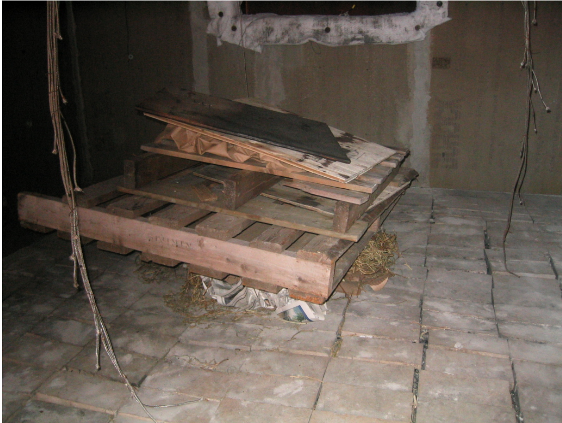
Figure 3.5: Typical Fuel Load for Fire Experiments, Located on Burn Pad
