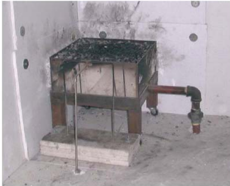
Figure 2.6: LPG Burner used in Room Fire Experiments at the University of Canterbury [27]
