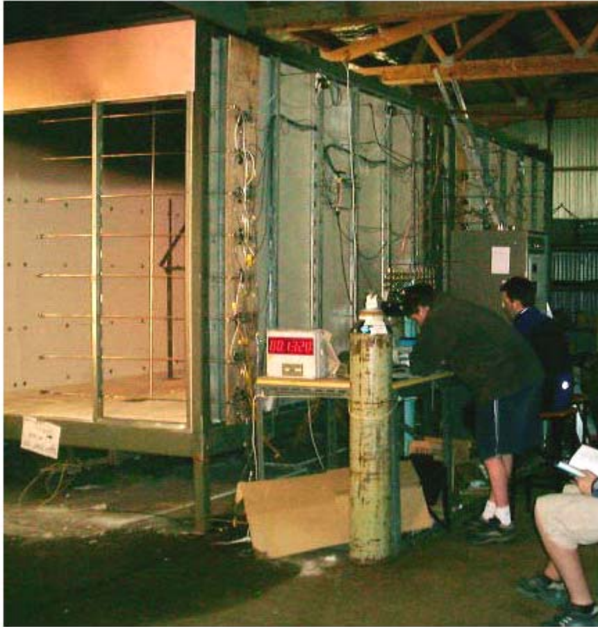
Figure 2.7: Experimental Set up of Two Room Enclosure at the McLean's Island Testing Facility [27]
