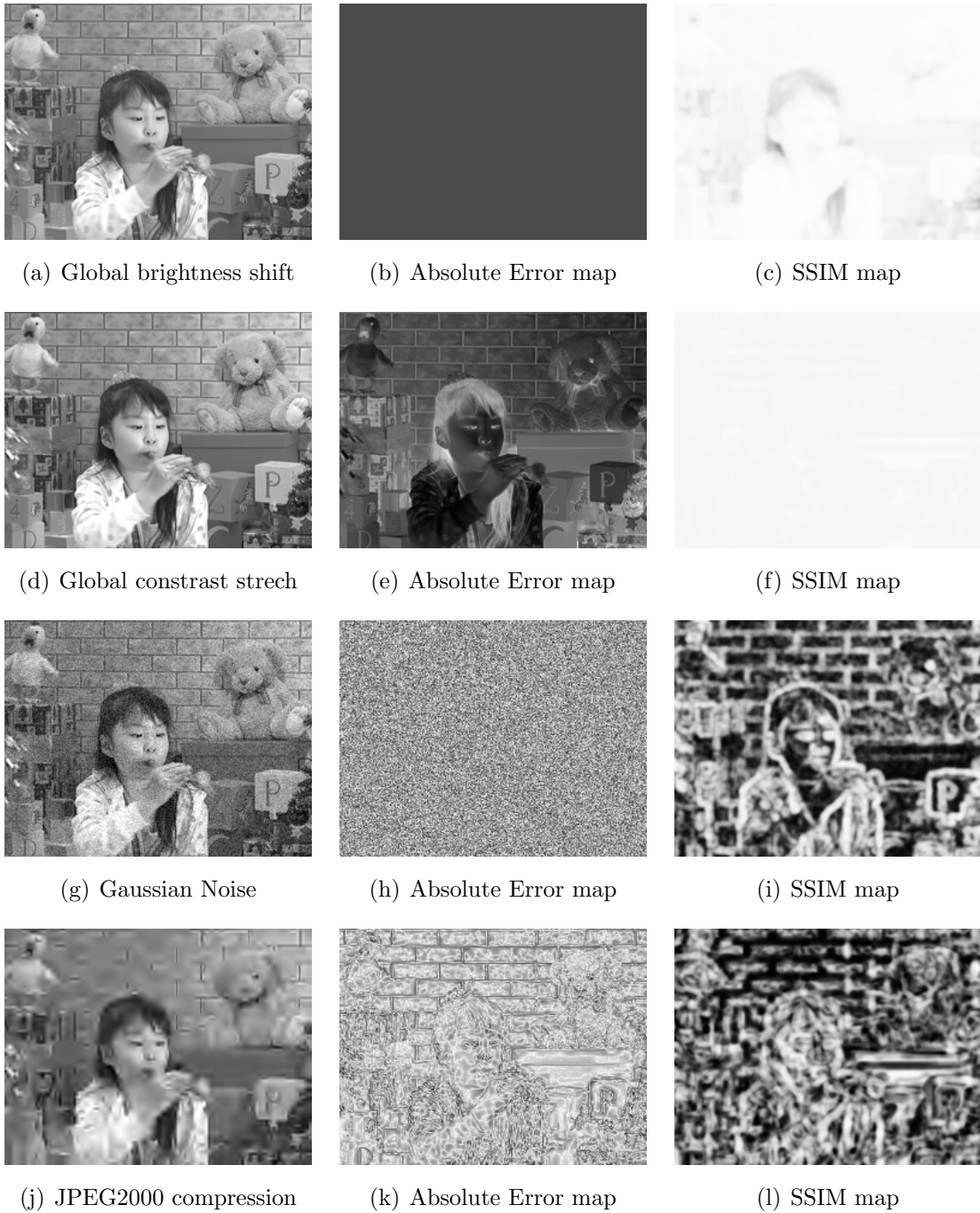
Figure 2.7: Comparison between MSE and SSIM local quality maps. In both maps, brighter indicates better local quality (or lower distortion)
