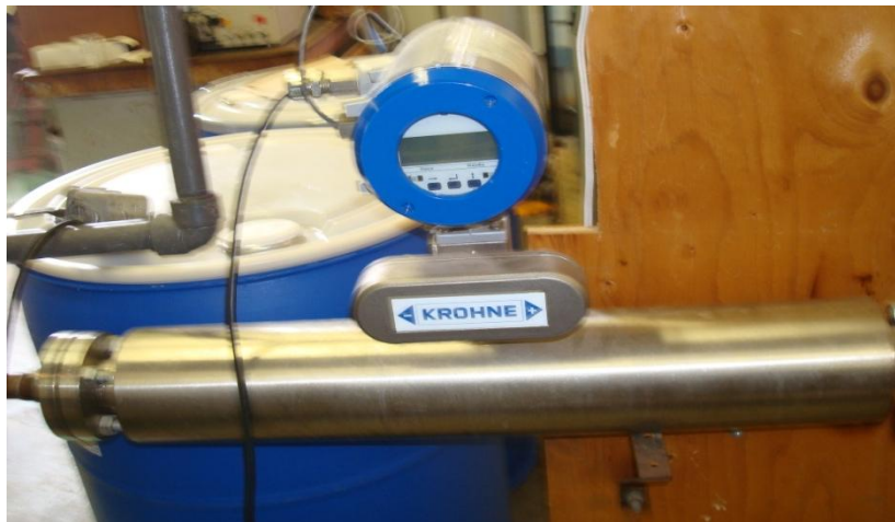
Figure 3.3 Picture of flow meter used
