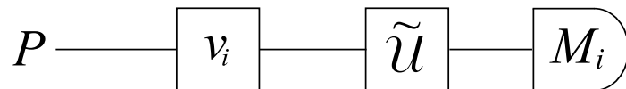
Figure 5.2: Modification of the circuit of Figure 5.1 by inserting the identity gate as \mathcal{U}^\dagger \circ \mathcal{U} , where \mathcal{U} is a Clifford and \tilde{\mathcal{U}} = \Lambda \circ \mathcal{U} is its faulty implementation. The measurement M_i = \mathcal{U}(P_i) is also a Pauli operator. This circuit is equivalent to that of Figure 5.1.
