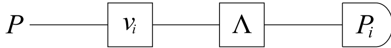
Figure 5.1: Circuit to measure t_i = \frac{1}{2^n} \text{tr}(\Lambda(P_i)P_i) , where P_i \in \mathcal{P}_n such that \text{wt}(P_i) = \omega . Here, P \in \mathcal{D} has weight \omega and, in the tensor product form, its identity terms are at the same positions than the identity terms of P_i . The operator v_i represents a sequence of single-spin \pi/2 such that P_i = v_i P v_i^\dagger .
