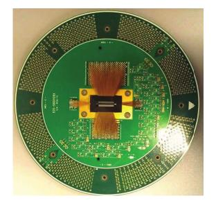
(a) A probe card with cantilever pins.
