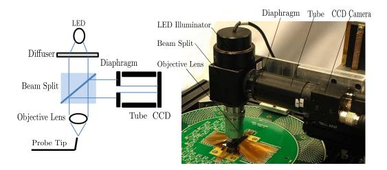
Figure 3.2: Configuration of the machine vision.
