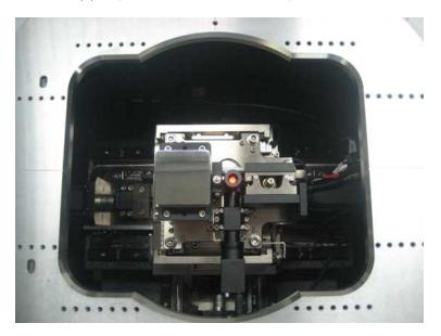
(b) The main part of a probe card analyzer.
