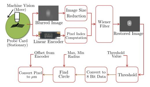
Figure 4.1: Real-time Image Processing Algorithm
