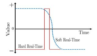
Figure 2.5: Value function for soft and hard real-time [41]
