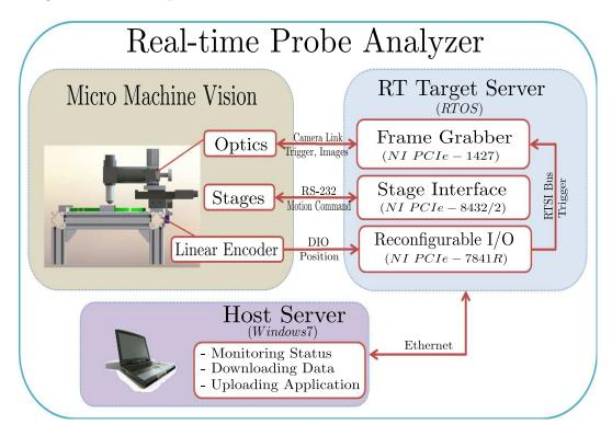
Figure 3.5: Configuration of realtime controller.
