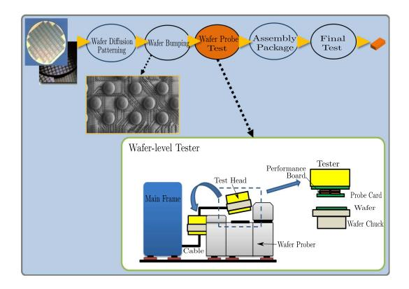
Figure 2.1: Schematic of the wafer-level test
