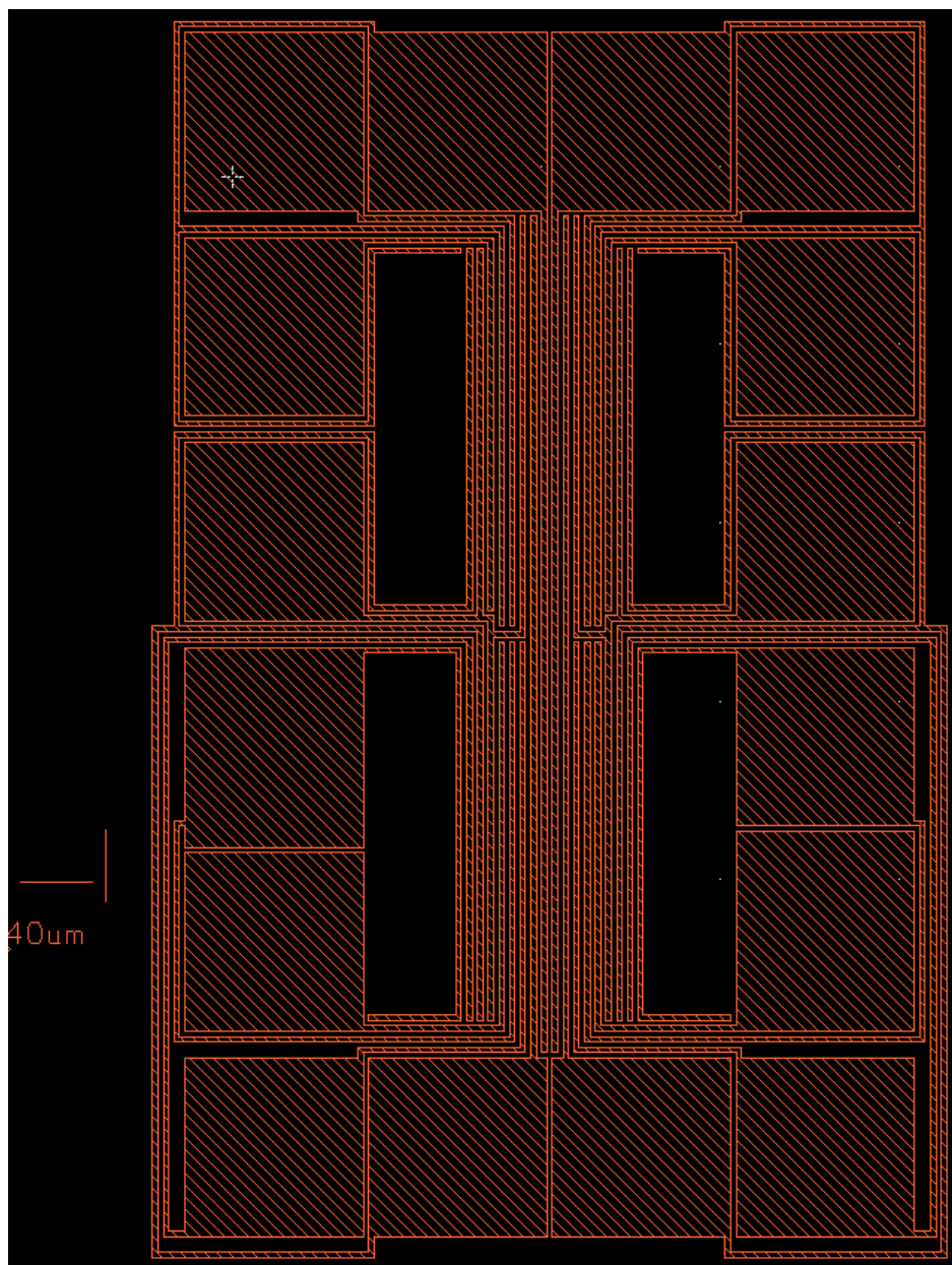
Figure 2.4: An example of a pattern invented to increase finger-area to pad-area ratio; this pattern has a ratio of 0.2. In the end however fabrication proved difficult and long fingers proved disastrous with silver particles shorting the electrode. For these reasons the design was never utilized
