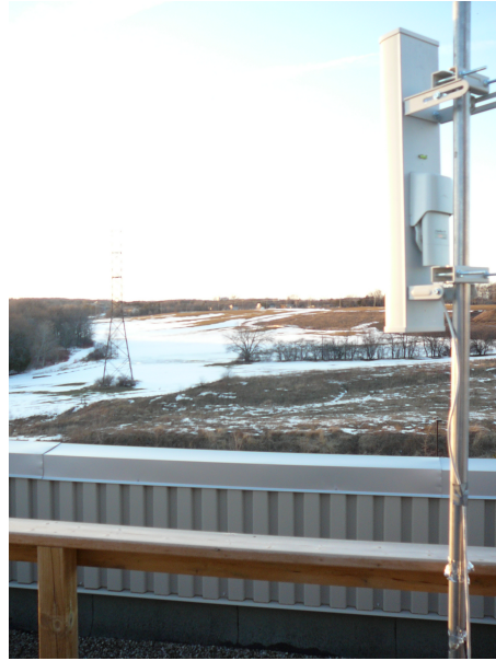
Figure 4.5: The Rocket M attached to the Airmax Sector antenna aiming out towards the two trailers. The antenna covered 120 degrees which easily encompassed the two trailers that required a classical data link.
