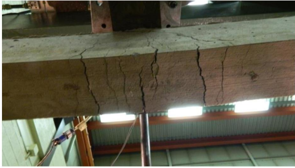
Figure 4-29: Bottom crack pattern
