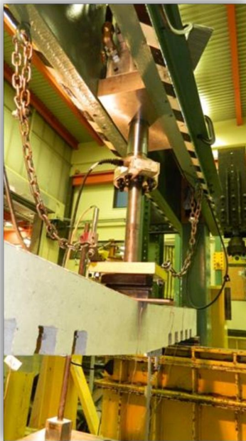
Figure 3-15: Testing specimens with hydraulic frame under point load
