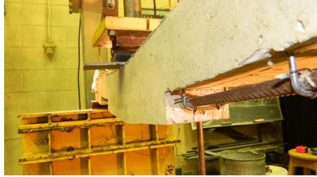
Figure 4-30: Testing beam under single point load
