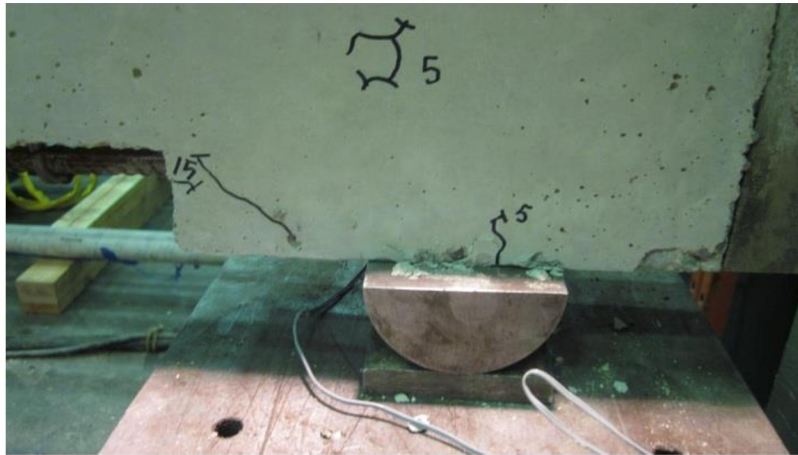
Figure 4-36: Beam support in specimen 6
