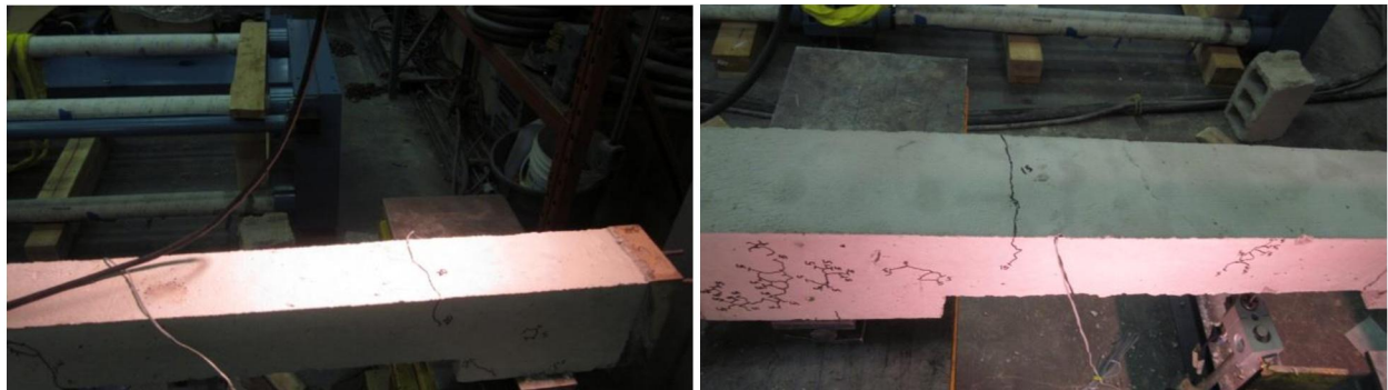
Figure 4-37: Crack on top face for specimen 6
