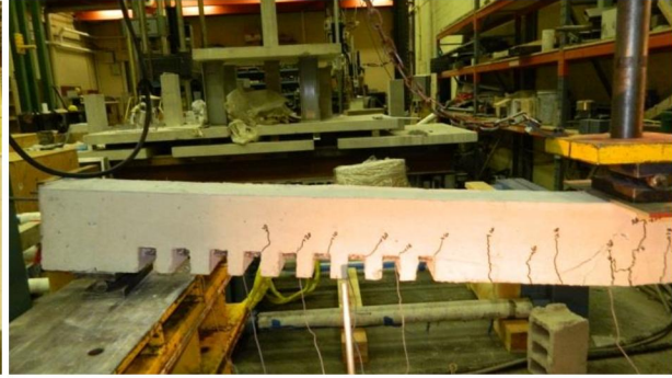
Figure 4-58: Flexural crack in specimen 9
