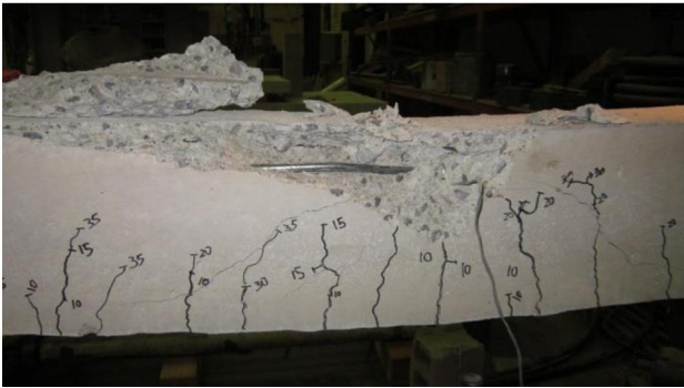
Figure 4-79: Concrete spalling in compression zone
