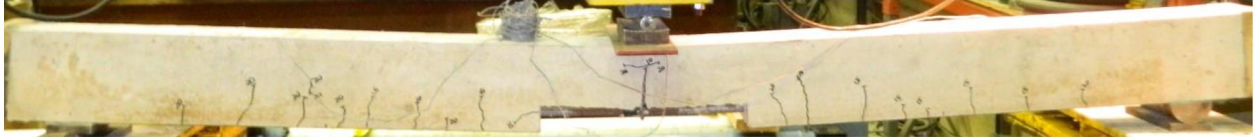
Figure 4-11: Crack pattern for specimen 2
