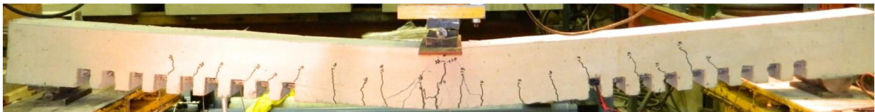
Figure 4-60: Crack pattern for specimen 9
