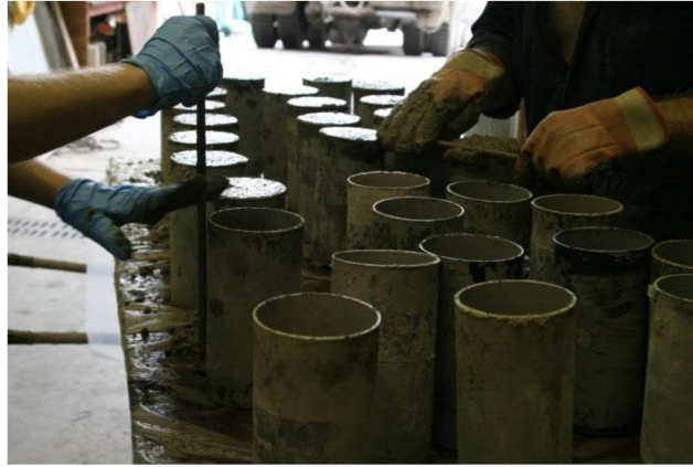
Figure 3-7: Casting cylinders for concrete compression test
