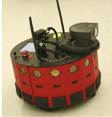
Figure 6.15: The MagellanPro mobile robot hardware platform provides actuators and sensors to carry out specific actions based on an understanding of human expression.
