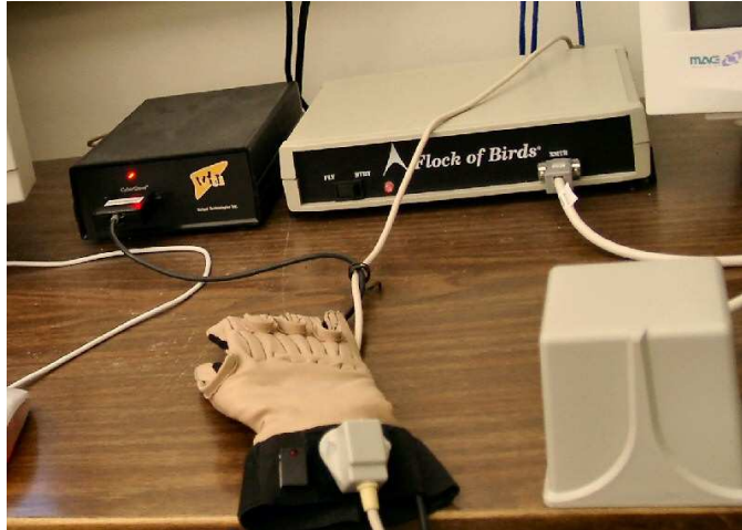
Figure 3.5: The Flock of Birds uses the DC pulsed electromagnetic source in the lower right corner together with the small directional sensor attached to the base of the glove to simultaneously determine 3D position and orientation. The CyberGlove uses strategically placed resistive bend sensors to measure hand and wrist joint angles. Hardware controllers for both devices are shown at the top, communicating with the computer over dedicated serial connections.
