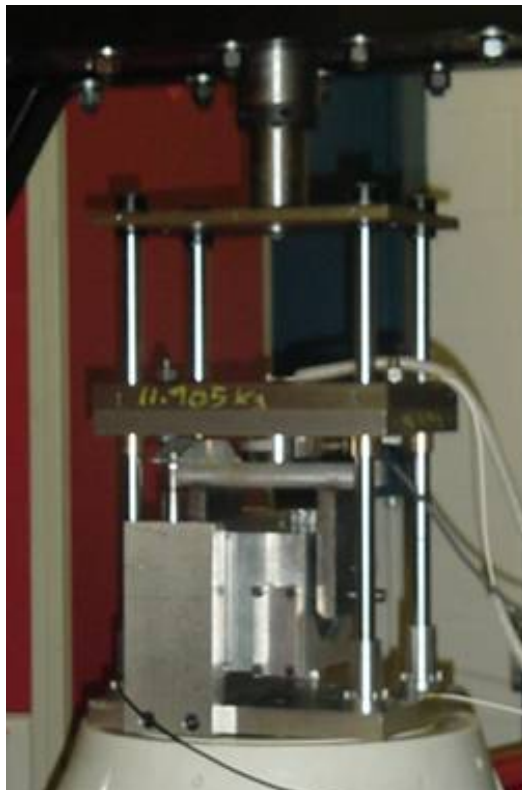
Figure 4-12: The MR valve set up used to conduct base excitation experiments
