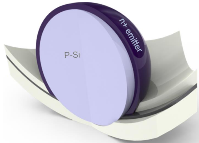
Figure 4.1: 3D schematic of a silicon sphere with diffused emitter thermally bonded to aluminum foil.
