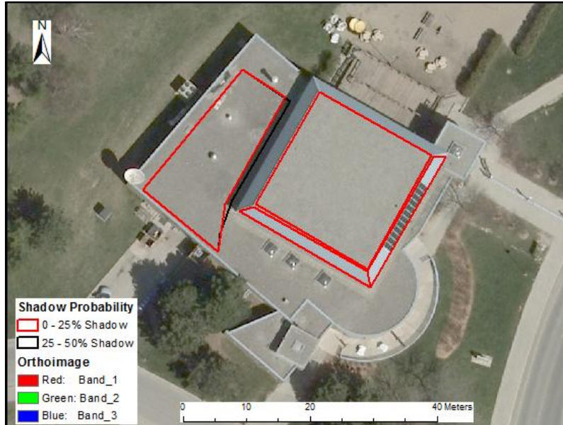
Figure 5.23 - Areas on FED Hall roofs with less than 25% and 50% of shadow risks overlaid on an orthoimage
