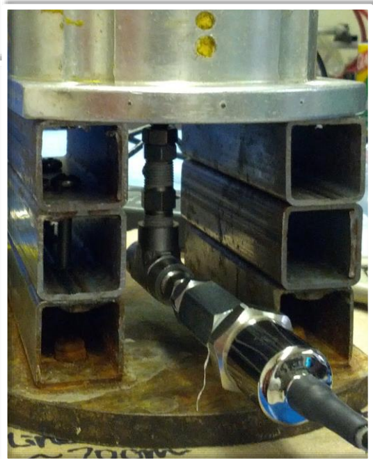
Figure 19: Specimen with the bore-screw pressure sensor system in the material testing system (top). Each specimen was mounted on a raised platform to provide clearance for the pressure sensor system at the bottom (bottom two pictures)
