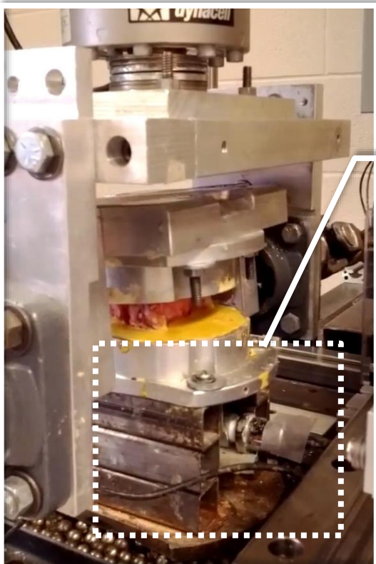
Figure 19: Specimen with the bore-screw pressure sensor system in the material testing system (top). Each specimen was mounted on a raised platform to provide clearance for the pressure sensor system at the bottom (bottom two pictures)
