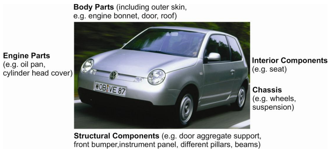
Figure 2-2: Magnesium sheet has been used in the VW-Lupo for automotive lightweight construction [14].
