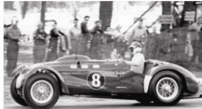
Series sports car Allard (1955) Car body out of Mg-sheet (thickness: 1.3 to 2 mm); Global weight (including doors and bonnet): 64 kg
