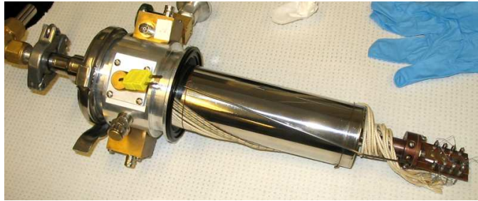
Figure 3.17: Dewar and sample holder used to hold sample for Hall effect measurements
