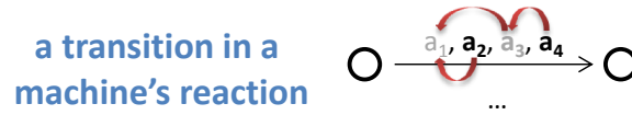
Figure 3.25: A transition involving preemptive actions: non-preemptive actions are not in bold (e.g., a_1 ), preemptive actions are in bold ( a_2 , a_3 , a_4 ), a red arrow goes from a preemptive action to its target action, and a preempted action is in gray.
