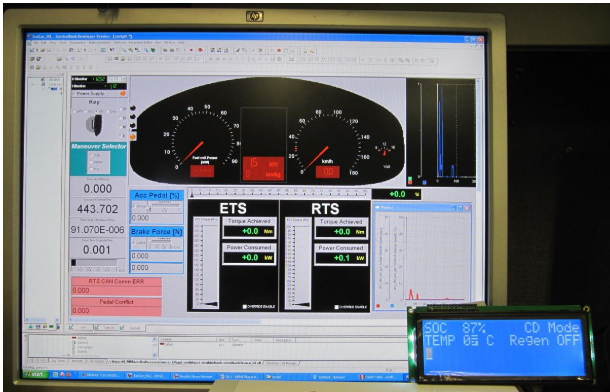
Figure 47: PC interface for the EcoCAR HIL setup
