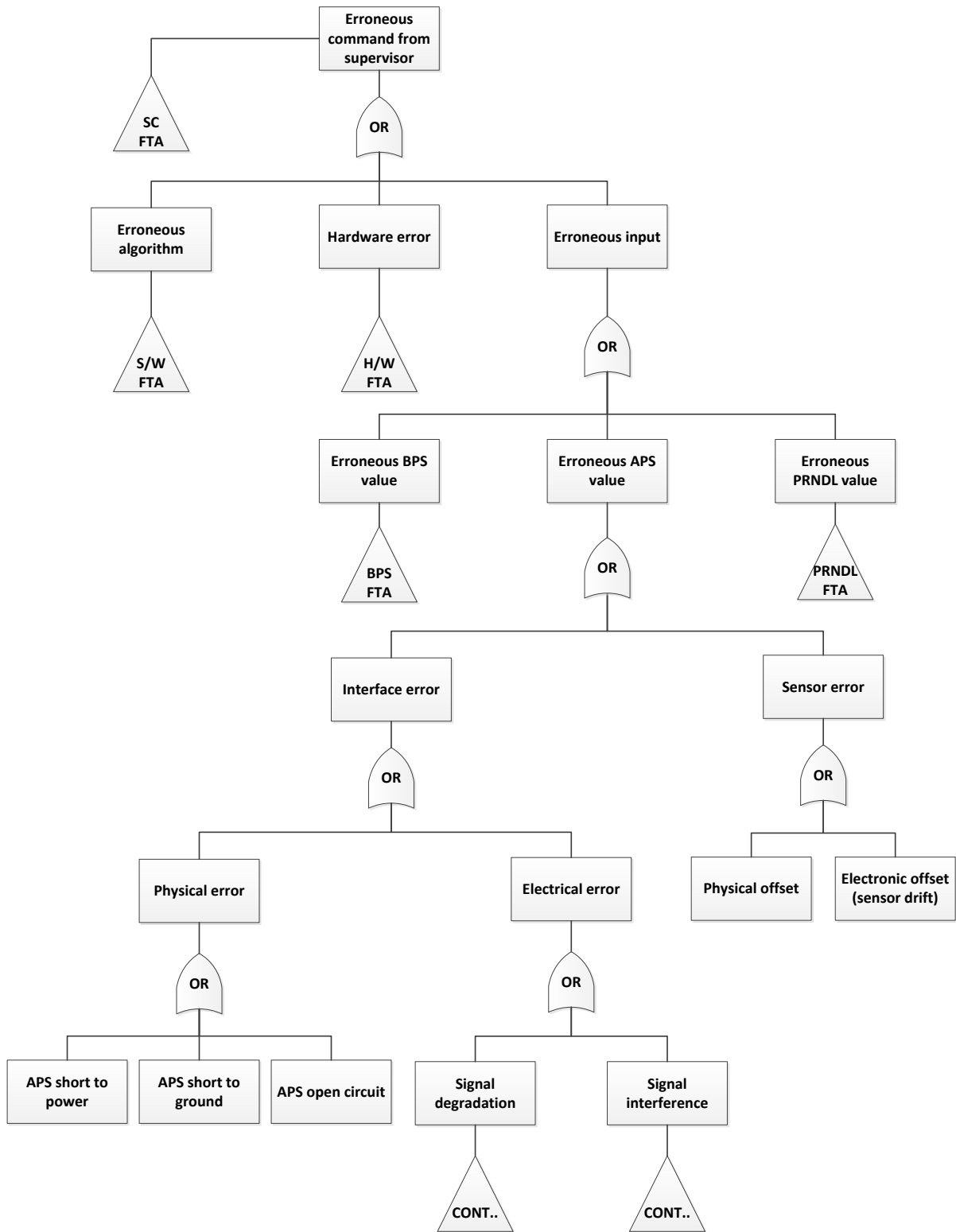
Figure 41: Fault tree for supervisory controller erroneous torque request
