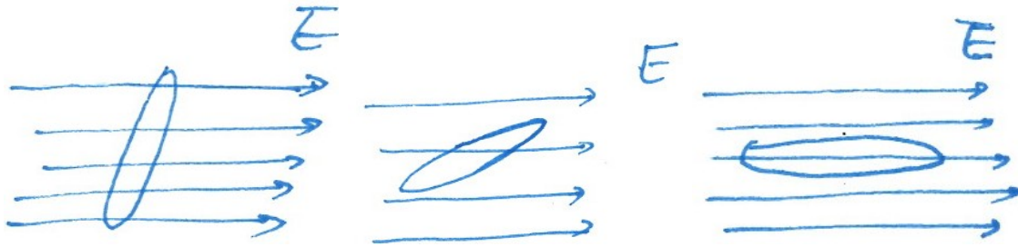
Figure 1.9: Schematic of an LC molecule, or mesogen, rotating in response to an electric field.
