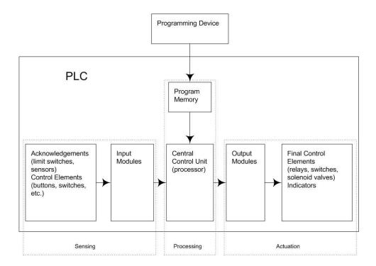
Figure 3 - Programmable Control (adapted from (Soloman 1994))
