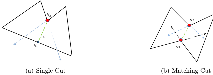
Figure 2.2: Two types of cuts possible in a non-convex polygon. Here, red dots represent an NCV. Green dashed lines represent an added cut edge. Dotted lines represent each vertex’s cone of bisection.
