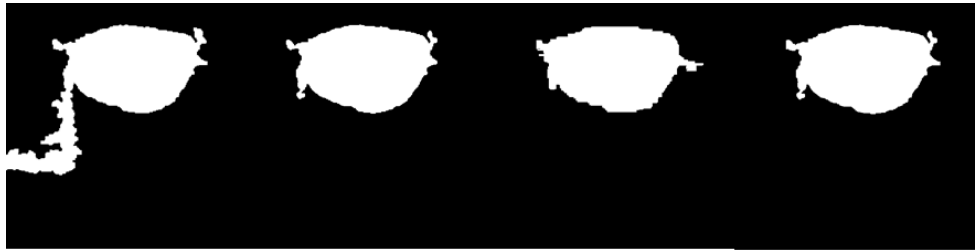
Figure 4.5: Sample results: (from left to right) results for Niblack, SRM, and RG and for all three fused by STAPLE. Note that the result of the fusion correctly reflects the fact that SRM is the best overall method based on the experiments.
