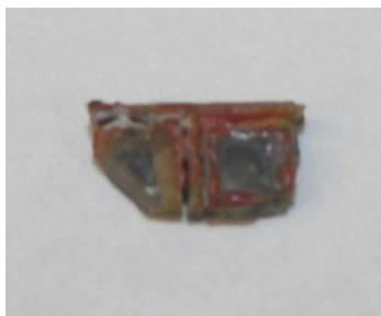
Figure 26: A square that was laser machined from the piezoelectric material using high power settings.
