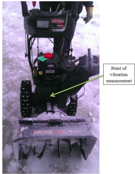
Figure 4-3: Snow blower Vibration Measurement location
