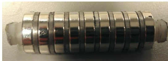
Figure 4-13: Mover consisting of magnet, iron pole, plastic nut and threaded rod
