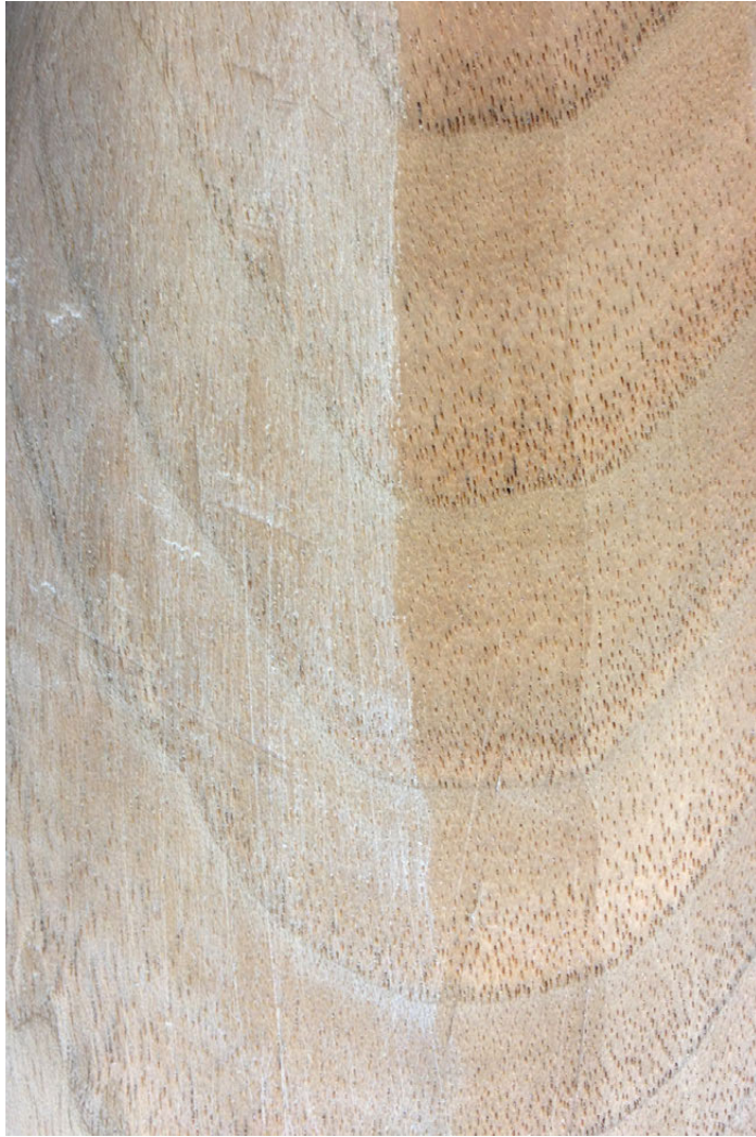
Figure 013 [Left] Sanded Wood Surface, [Right] Hand-planed Wood Surface
