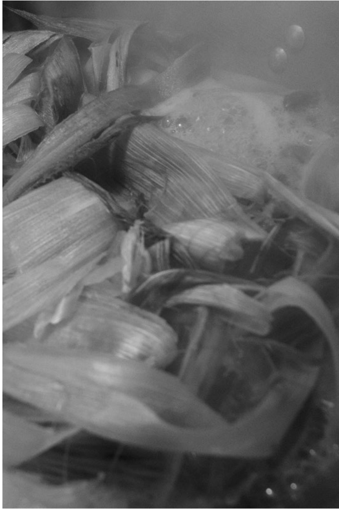
Figure 007 Cooking Fibre with Soda Ash
