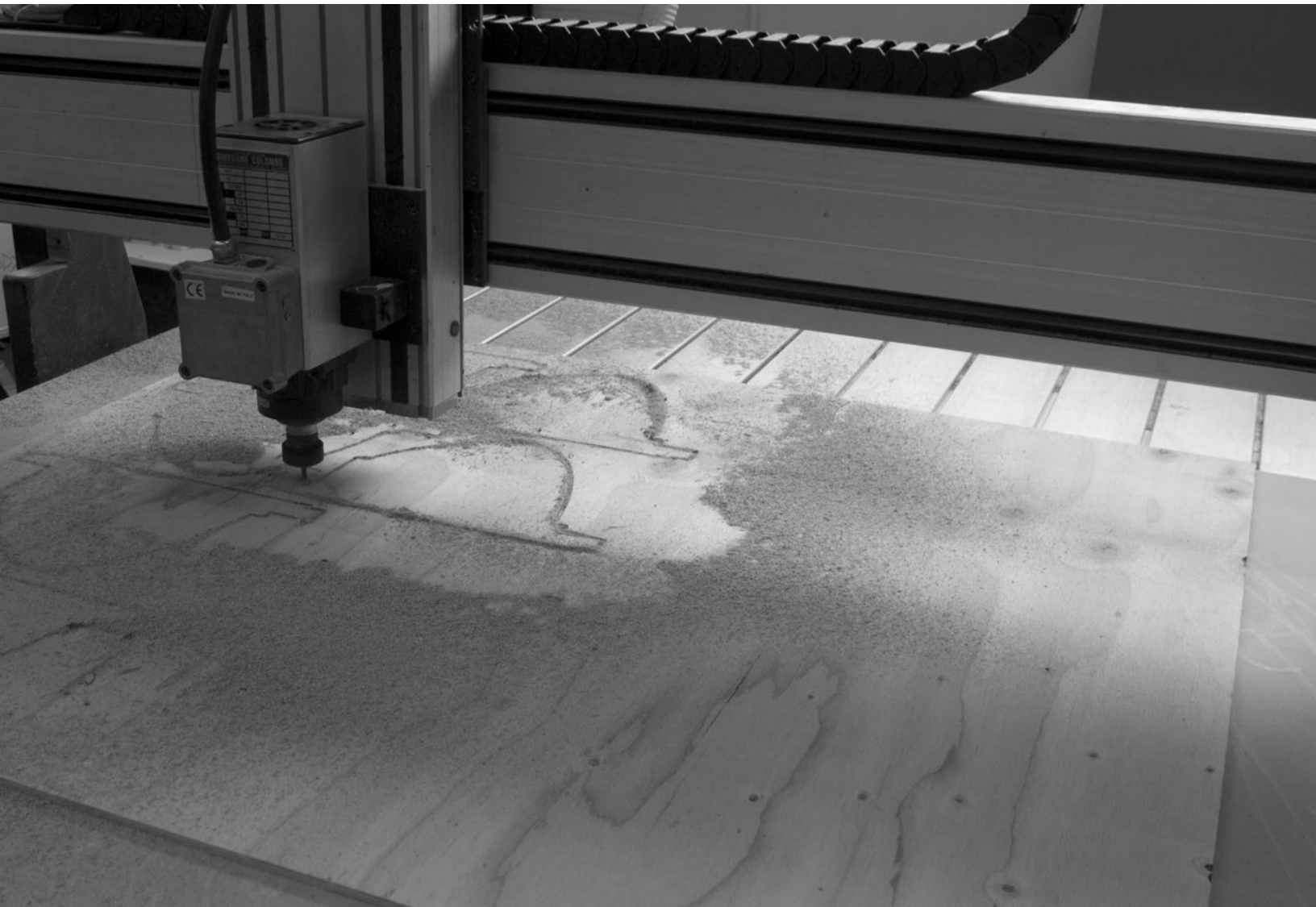
Figure 178 Using the CNC Router
