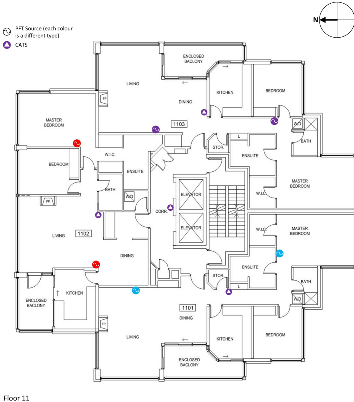
Figure 7-12: Layout of PFT testing equipment on Floor 11 of the case study building
