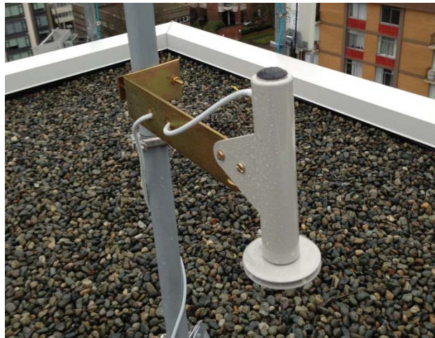
Figure E-4: Photo of exterior pressure for roof mounted on weather station tripod
