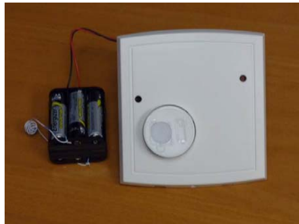
Figure 7-22: Front face of a typical data acquisition unit used at the case study building with the faceplate cover installed showing holes on the front of the cover to expose the temperature and relative humidity sensors (left) and pressure tube (top right)
