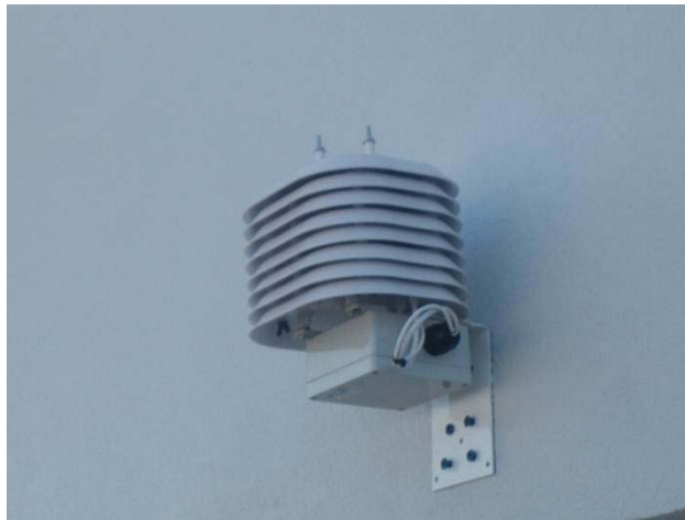
Figure E-1: Photo of SMT-A3 unit in a waterproof exterior enclosure for use outside as the ROOF and GROUND units which include a shroud on top containing the temperature, relative humidity, and CO2 sensors.
