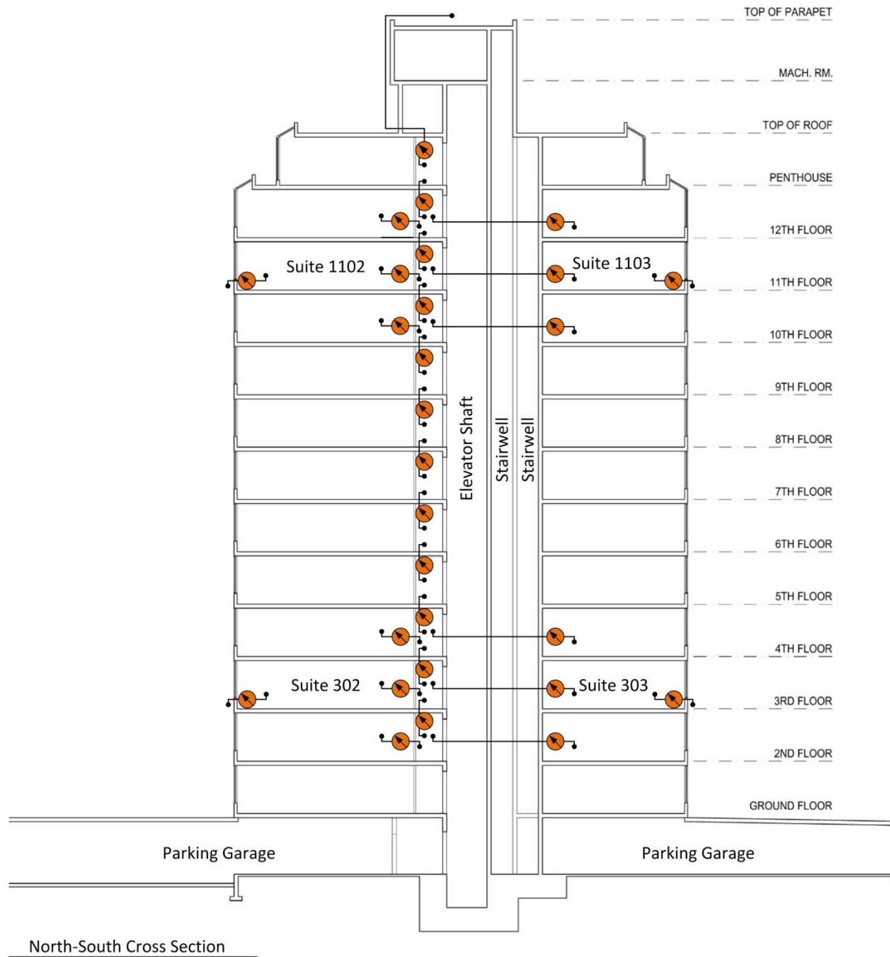
Figure 7-28: North-south cross-section of the case study building illustrating how the pressure measurements are linked
