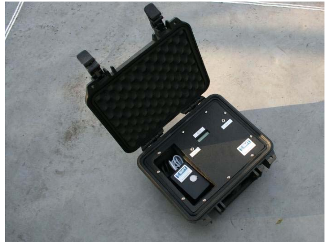
Figure E-2: Photo of SMT-A3 unit installed in a waterproof outdoor case for use as FLOAT05 and FLOAT06 units with sensors attached via leads.
