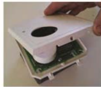
Hook faceplate on top and push down.
