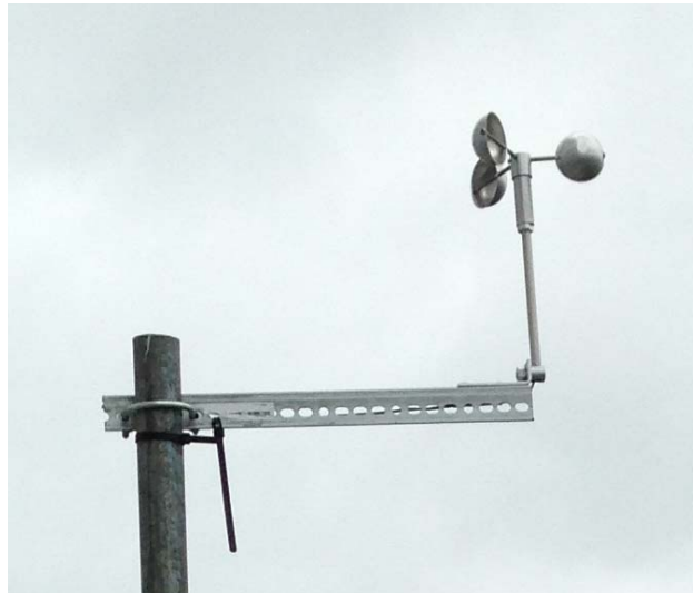
Figure 6-9: Typical hemispherical cup type anemometer used for measuring wind speed
