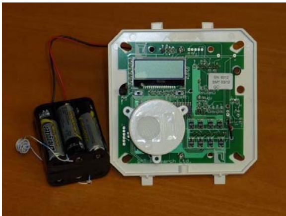
Figure 7-21: Front face of a typical data acquisition unit used at the case study building showing the LCD screen to interact with the unit (top left), the carbon dioxide sensor (bottom left, round and white), and battery pack left
