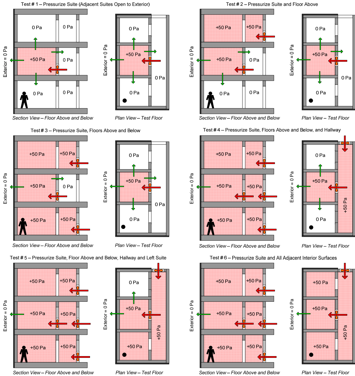
Figure 6-6: Schematic showing sequentially neutralized pressurization/depressurization airtightness testing steps for a typical multi-unit residential building (Finch, Straube, & Genge, 2009)
