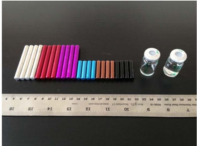
Figure 7-10: PFT sources used at the case study building. Each colour is a different PFT tracer and the glass vials are “mega” sources of a distinct PFT used in the MAU.
