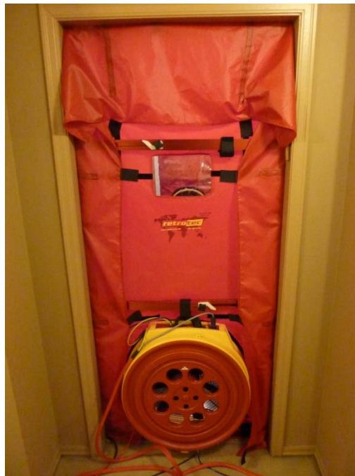
Figure 6-5: Typical Canvas Fan-Door Used for Airtightness Testing
