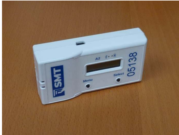
Figure E-3: Photo of typical SMT-A2 unit used for FLOAT01, FLOAT02, FLOAT03, and FLOAT 04
