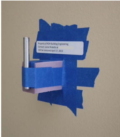
Figure C-1: Photo of typical source installation using an extruded polystyrene block to space off the wall with a label to identify the source
