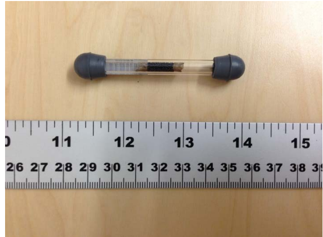
Figure 7-11: Typical CATS used for PFT testing at the case study building
