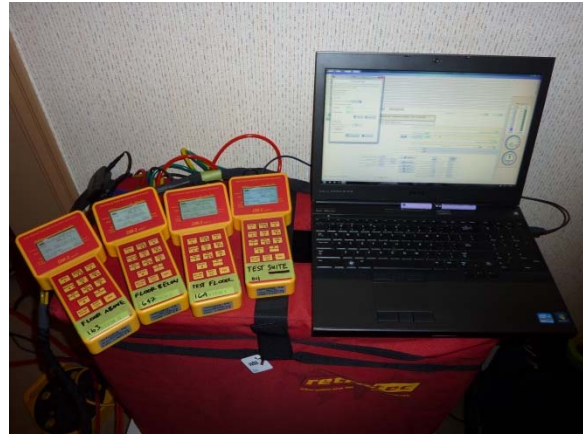
Figure 7-20: Laptop and four digital manometers used for controlling the airtightness testing fans and for making the pressure and airflow measurements during the test
