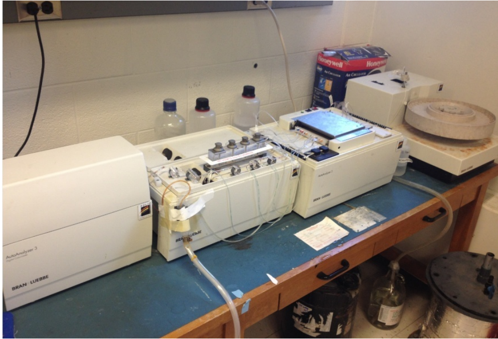
A4. Bran-Luebbe Auto Analyzer 3 for ammonia measurement
