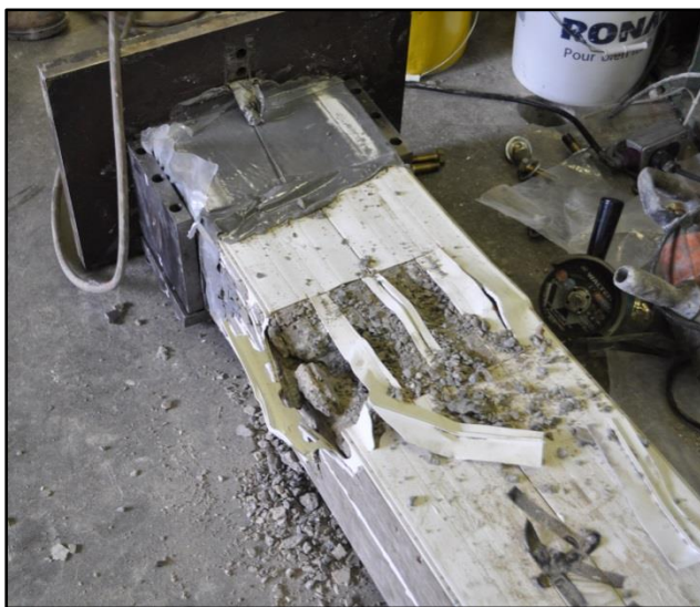
b- Confined specimen after failure
