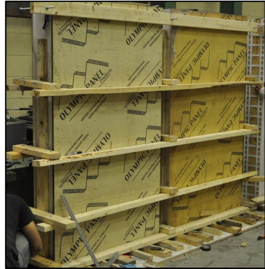
b- Boxes for the control specimens after bracing
