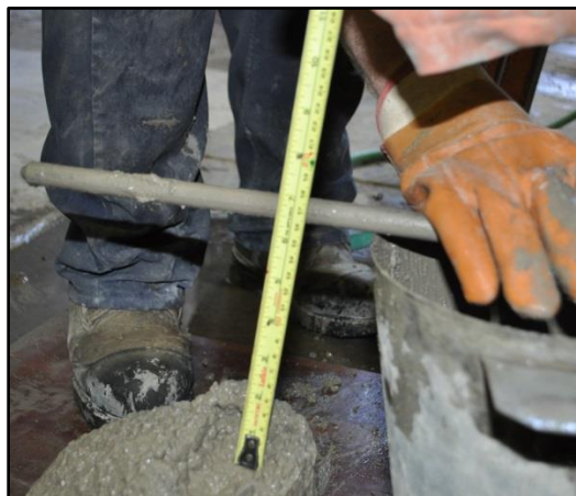
Figure 2.6 - Standard slump test
