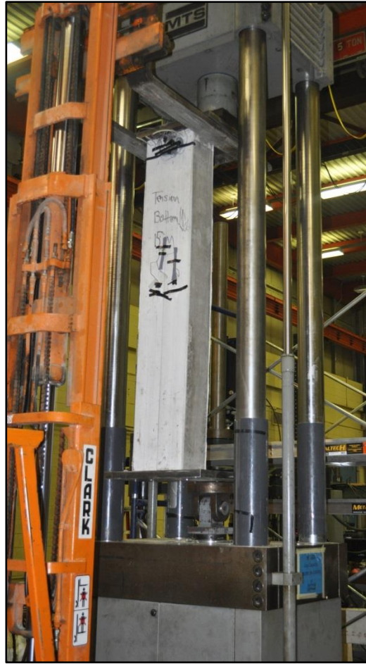
Figure 2.9 - Forklift placing the specimen inside the frame
