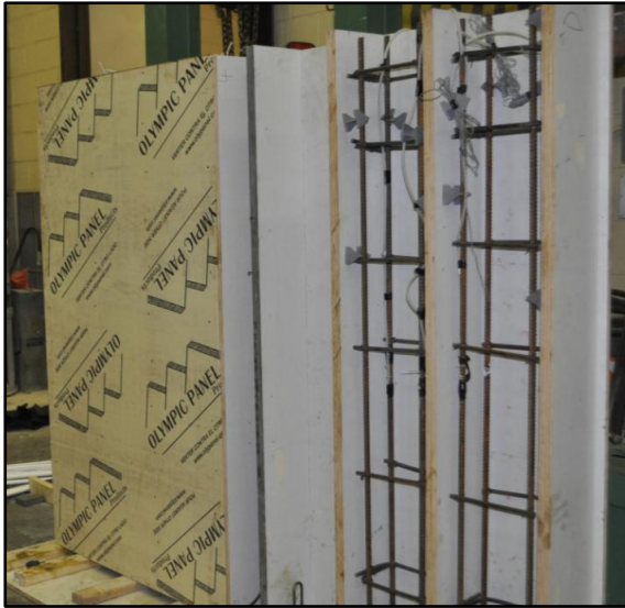
a- Boxes for the control specimens before bracing
