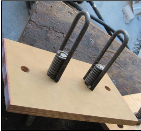
a- Top end plates with straight coil loop inserts
