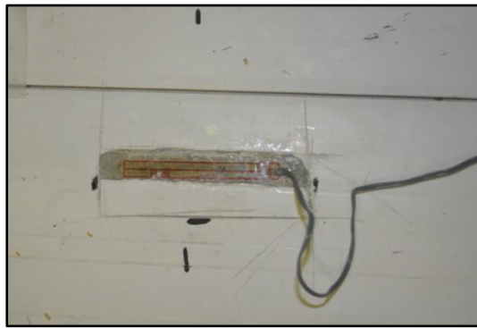
a- Strain gauge mounted on the concrete
