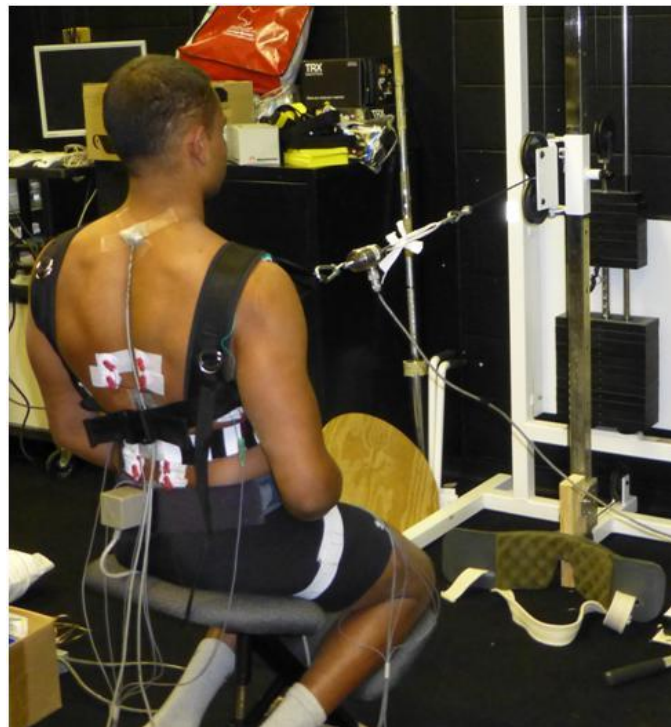
Figure 11: Active extension trial setup. The subject sits in a 'balans' chair used to foster a neutral spine and hip posture, loaded anteriorly with a 35 lb load. Applied moments were calculated based off the applied load and moment arm from the point of load application to the level of the L5.
