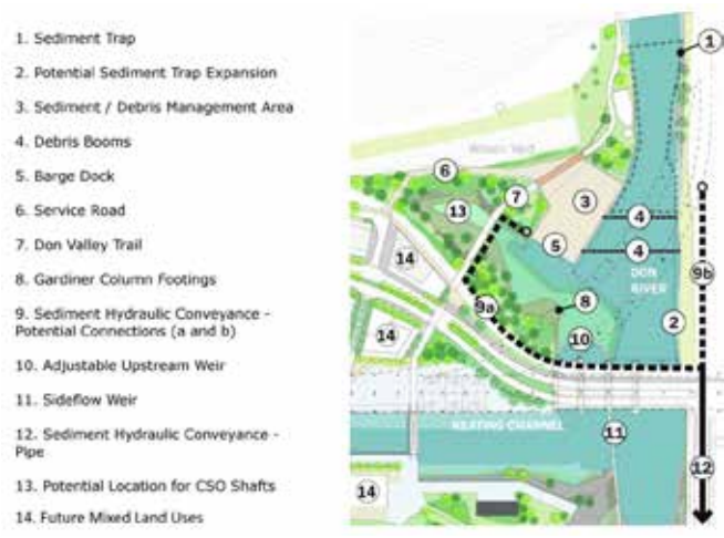
Fig. 3.32: Site plan of sediment traps and processing facilities for Lower Don Lands proposal.
