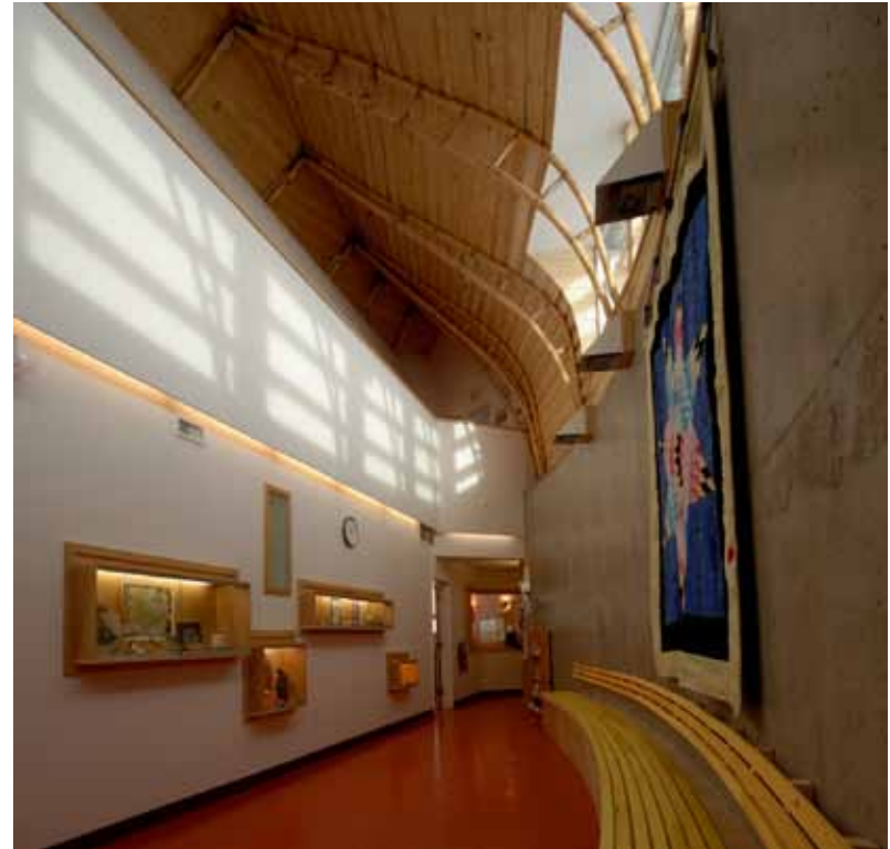
Fig. 4.31 - Reception area also acts as a gallery. The double-height hand plastered space provides naturally light and aids in the passive ventilation strategy.
