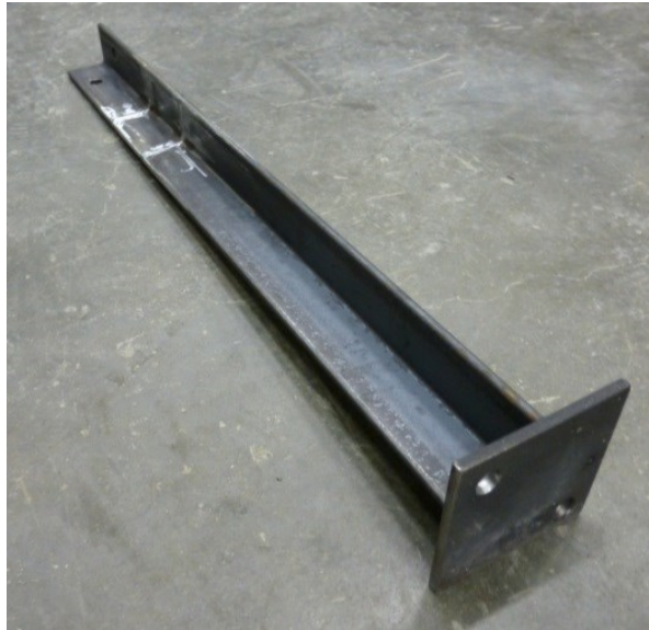
Figure 4-6: Structural testing rig legs
