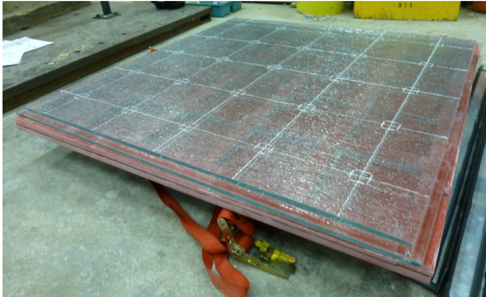
Figure 4-9: Structural testing load application points
