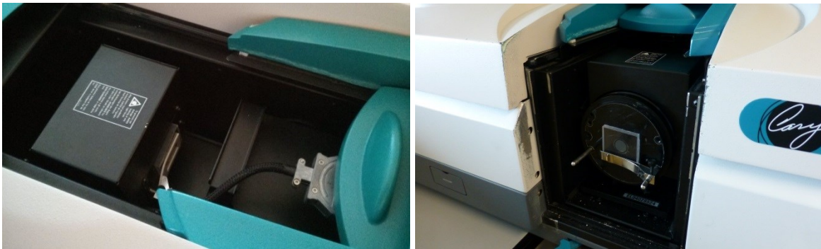
Figure 4-29: Sample positioning for transmissivity and reflectivity testing (left to right)
