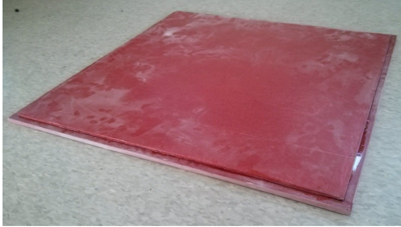
Figure 3-10: Base layer fiberglass epoxying
