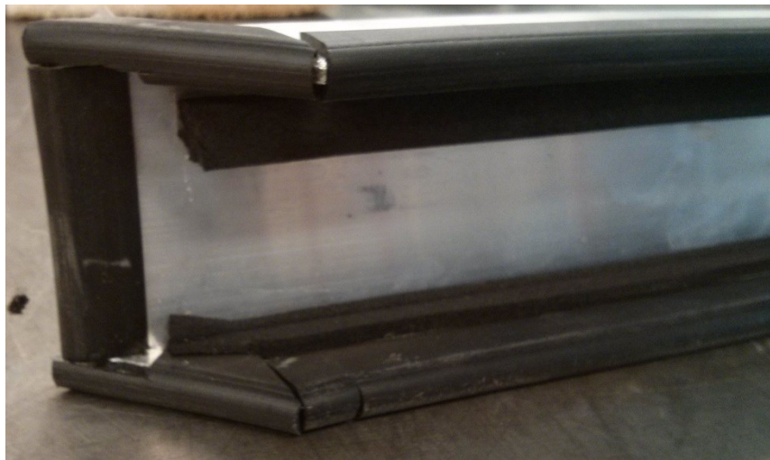
Figure 3-17: Housing frame with edge trim and foam inserts
