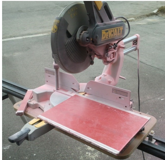
Figure 3-12: Optical rib cutting with a chop saw
