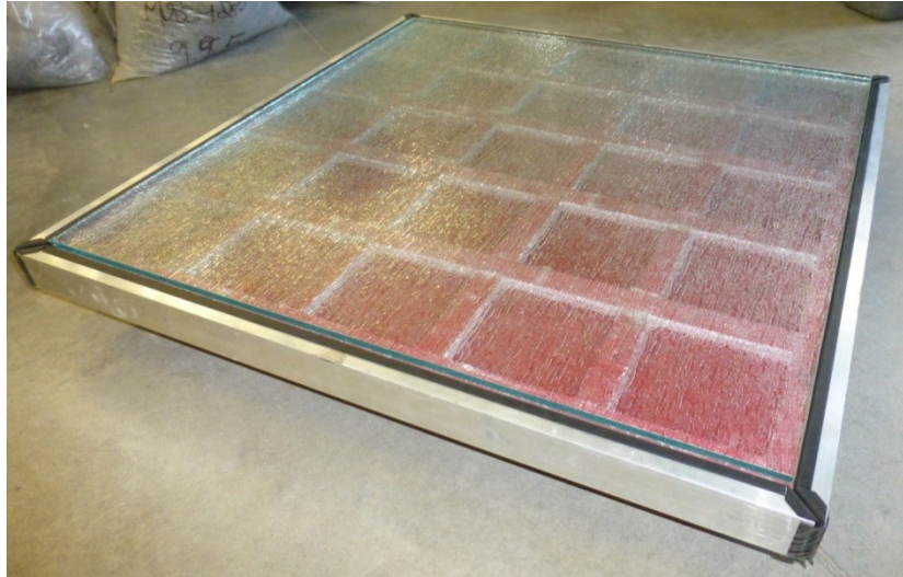
Figure 3-18: Completed structural solar road panel prototype
