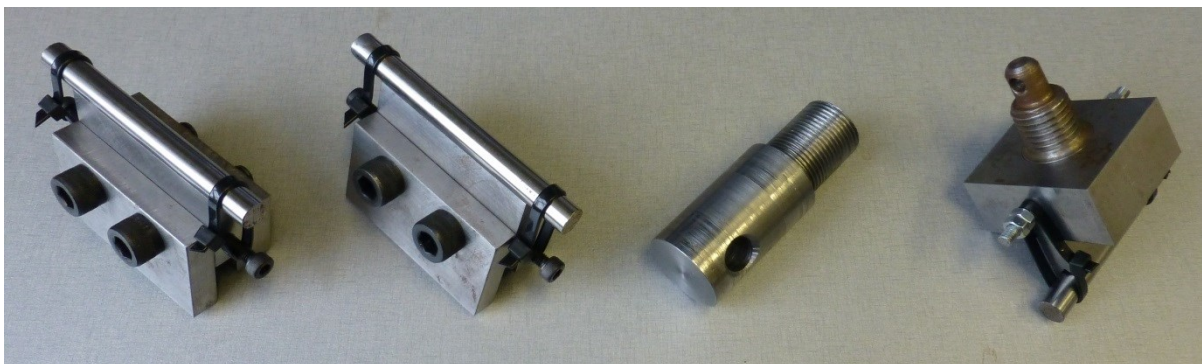
Figure 4-24: 3-point bending test support noses, base collar, and load nose (left to right)
