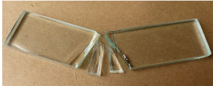
Figure 6-4: Typical glass 3-point bending test failure (Specimen G-15-US-3)
