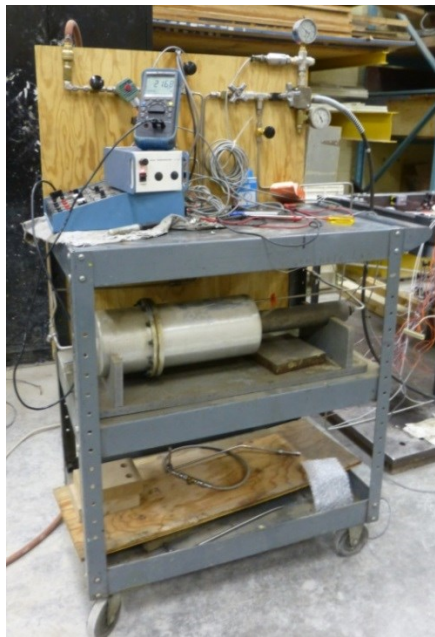
Figure 4-8: Structural testing air-over-oil system
