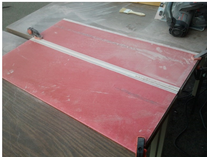
Figure 3-11: Optical layer fiberglass sheet trimming
