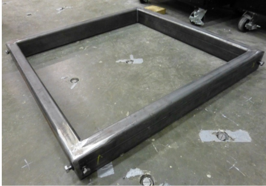
Figure 4-5: Structural testing rig loading ring
