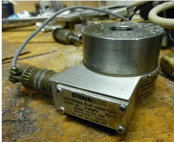
Figure 4-10: Structural testing load cell
