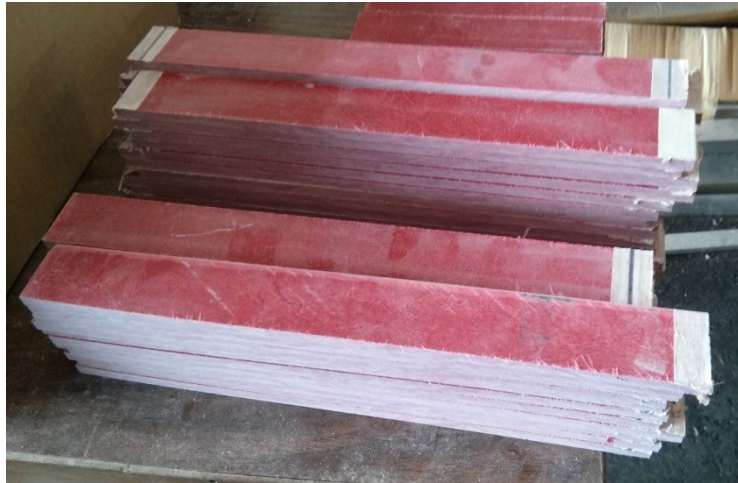
Figure 3-13: Fiberglass ribs marked for trimming
