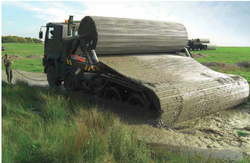
Figure 2-4: Faun Trackway heavy ground mobility system installation (FAUN, 2012)
