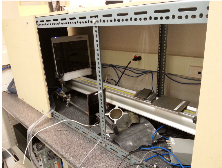
Figure 4.3: FLAATZ-330N set up for DQE measurements.
