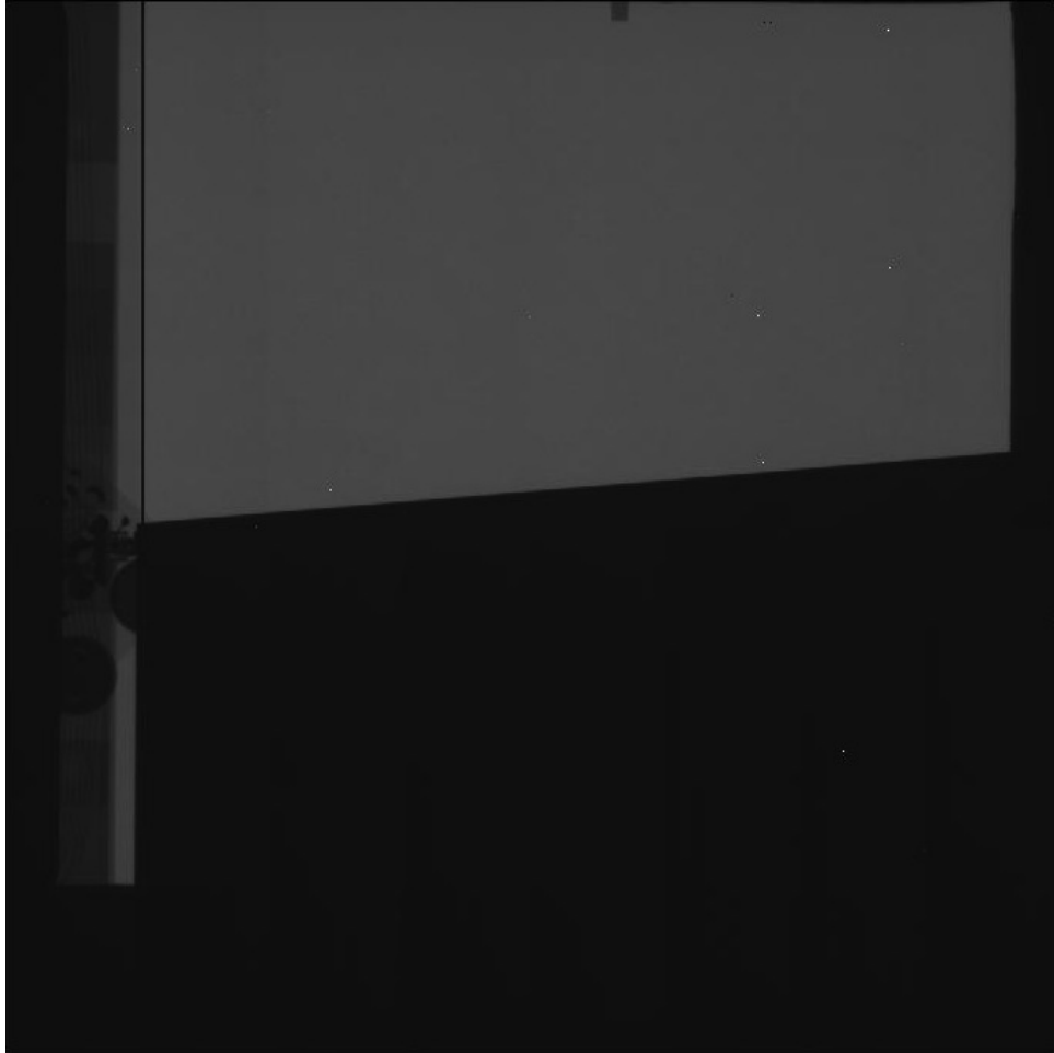
Figure E.2: Edge image for calculating MTF in the y-direction of the XRD0820.
