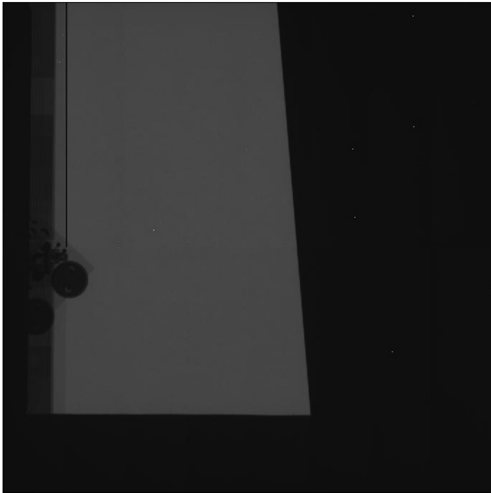
Figure E.1: Edge image for calculating MTF in the x-direction of the XRD0820.
