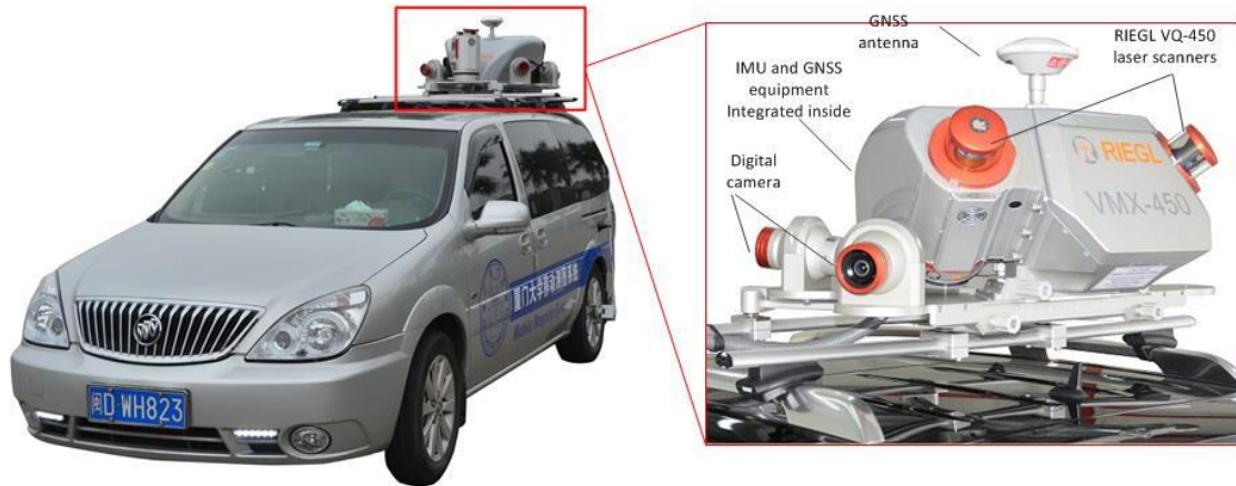
Figure 3.2: RIEGL VMX-450 system with an inset picture of the laser scanning and navigation system mounted on the roof rack.
