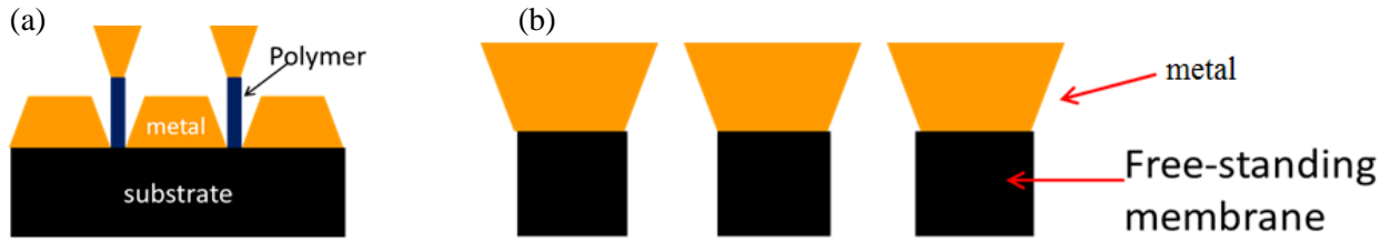
Figure 6.29 Schematic of a periodic array of tapered nan-hole array in Au film fabricate by (a) double lift-off process and (b) evaporation of Au onto the hole array patterned on a free standing membrane. The structures are illuminated by TM polarized light from glass side.
