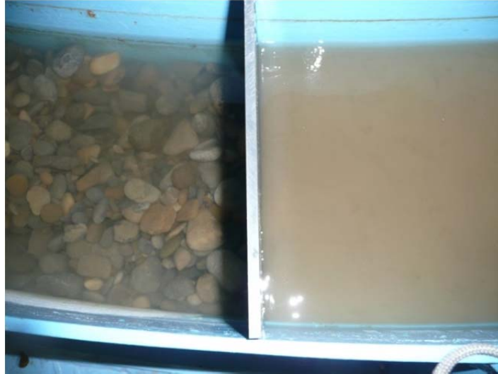
Figure 4.4 Resuspension of fines from the gravel bed (due to mechanical mobilization of the gravel bed). Left Cell is Undisturbed and Right Cell has been Mechanically Agitated.
