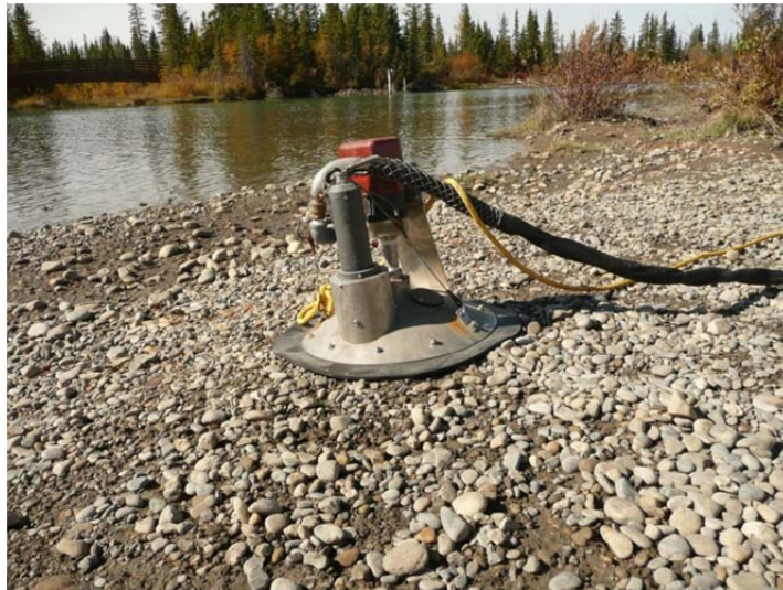
Figure 2.2 Inverted Cone Sampler used to Collect Cohesive Sediment and Water from the bed of the Elbow River.
