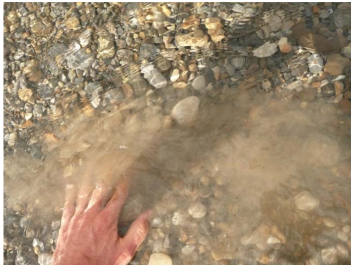
Figure 4.5 Mobilization of fine sediments through mechanical disturbance in the Elbow River bed.
