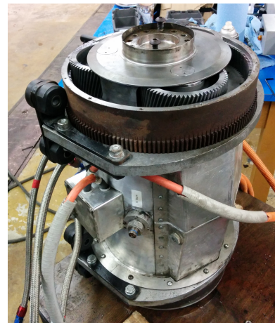
(b) Closeup of Motor Gearbox
