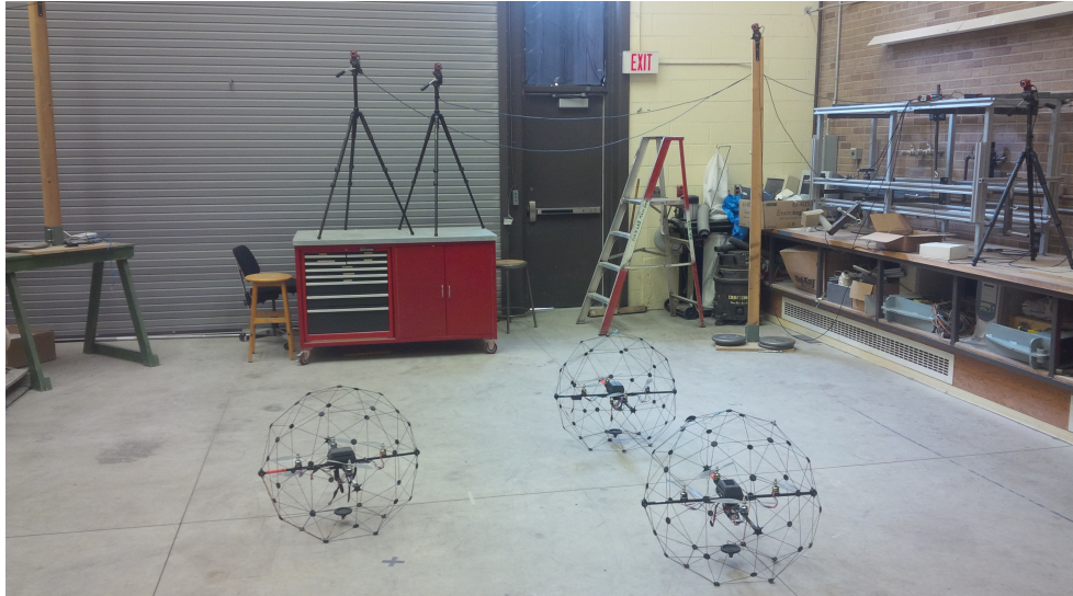
Figure 2.4: Multi-quadrotor Qball-X4 swarm system
