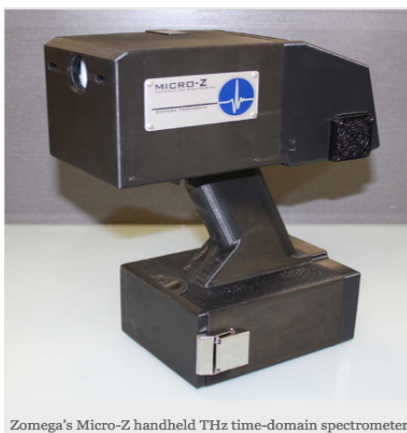
Figure 3.21. A real time terahertz TDS device for explosive identification 12 .
