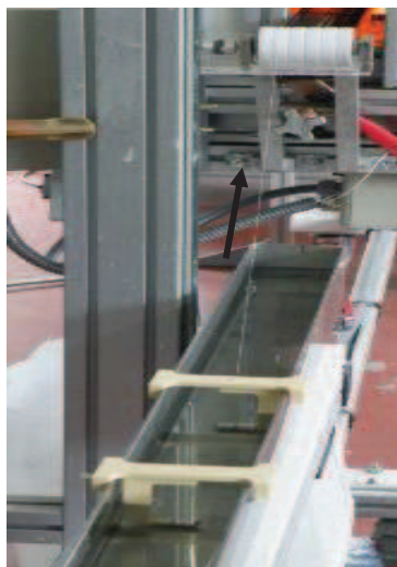
Figure 11. Picture of the fiber passing through the washing bath (aqueous solution containing sodium tetraborate at 0.1 mol.L -1 ).
