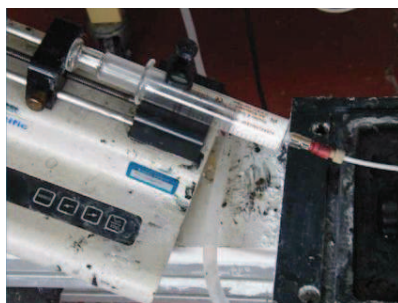
Figure 9. Picture of the syringe pump used for the injection of the starting solution in the coagulation bath.
