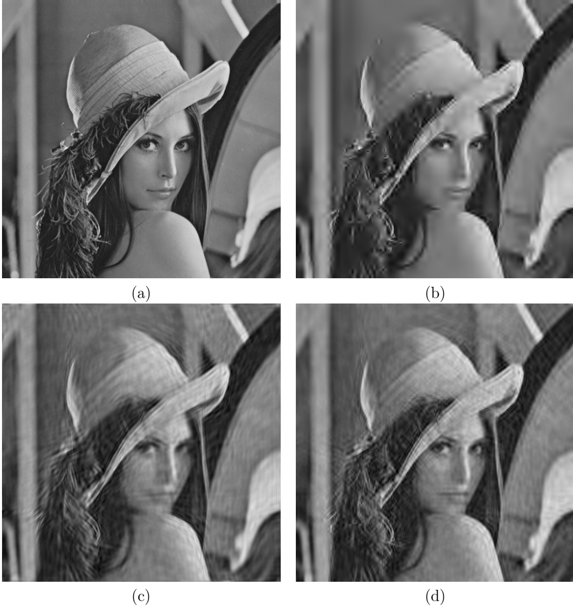
Figure 7.8: The Lena test image under severe compression. The original is shown in (a), and a compressed version using (b) Biorthogonal wavelets, (c) DOST, (d) DCST. The compressed versions retain only 1% of the original image's coefficients, and have mean-SSIM's of (b) 0.765, (c) 0.734, (d) 0.759.
